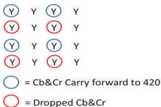
Figure 7-99. LDC YUV422 to YUV420 Conversion
