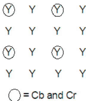
Figure 7-97. LDC Sample Grids for NV12
