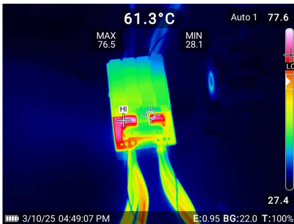
Figure 3-7. Thermal Capture (48V–12V, 1.1kW, 25°C Ambient, 29.5 Cubic Feet per Minute Airflow)
