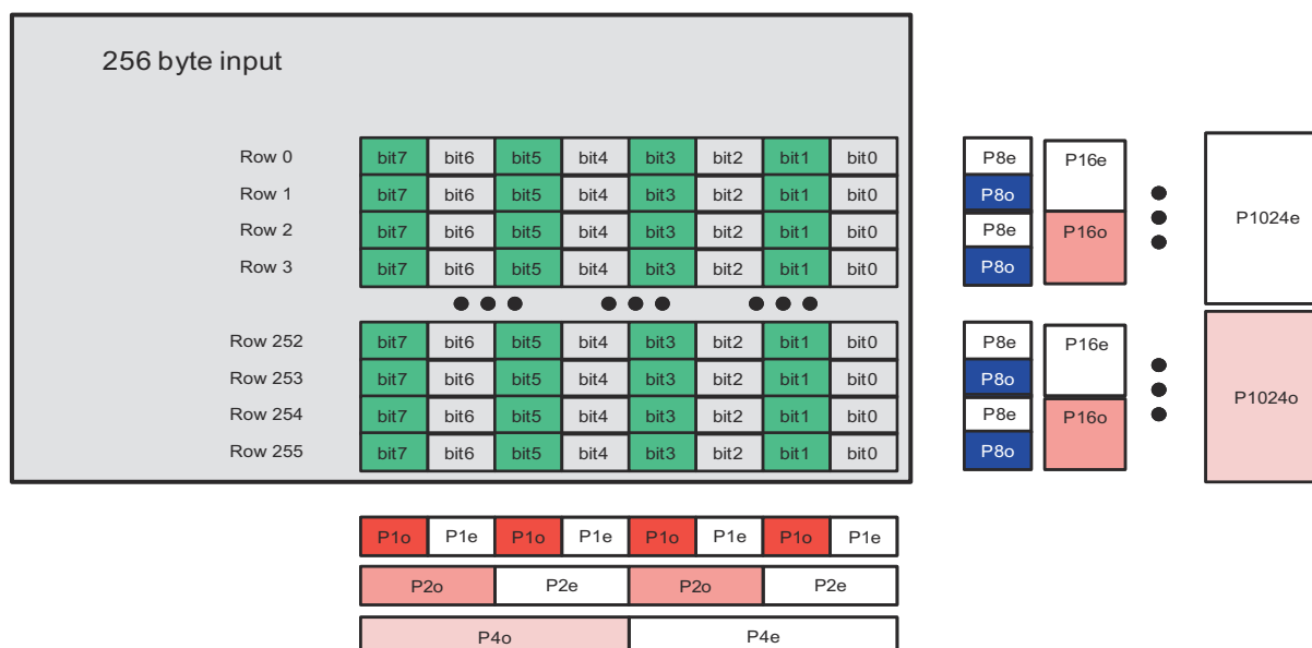
Figure 17-86. ECC Computation for a 256-Byte Data Stream (Read or Write)
