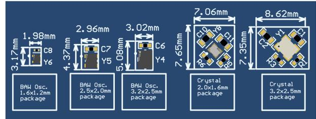
Figure 2. PCB Footprint Comparison of BAW Oscillator and Crystal
