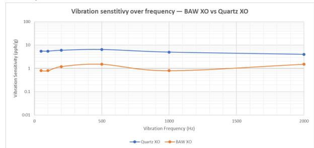
Figure 3. BAW Oscillator Vibration Sensitivity
