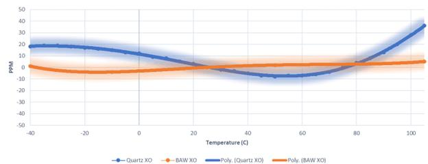
Figure 4. Temperature Stability Comparison of BAW Oscillator and Quartz
