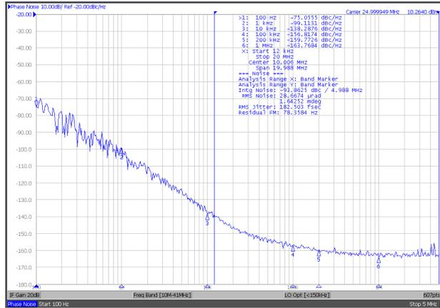
**Figure 5. LMK6C BAW Oscillator 25 MHz Phase Noise Performance**
