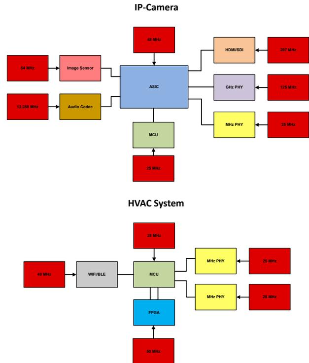
**Figure 6. Typical Block Diagrams of BAW Oscillator Used in Building Automation**
