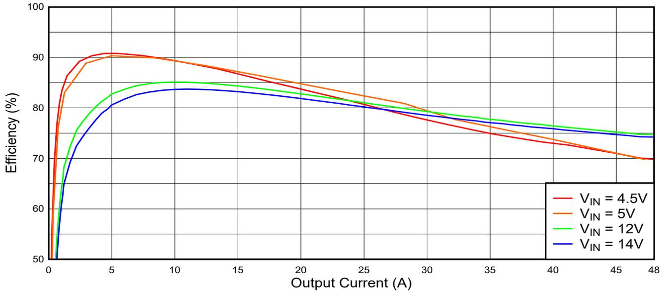
Figure 3-7. Efficiency FSW = 500kHz
