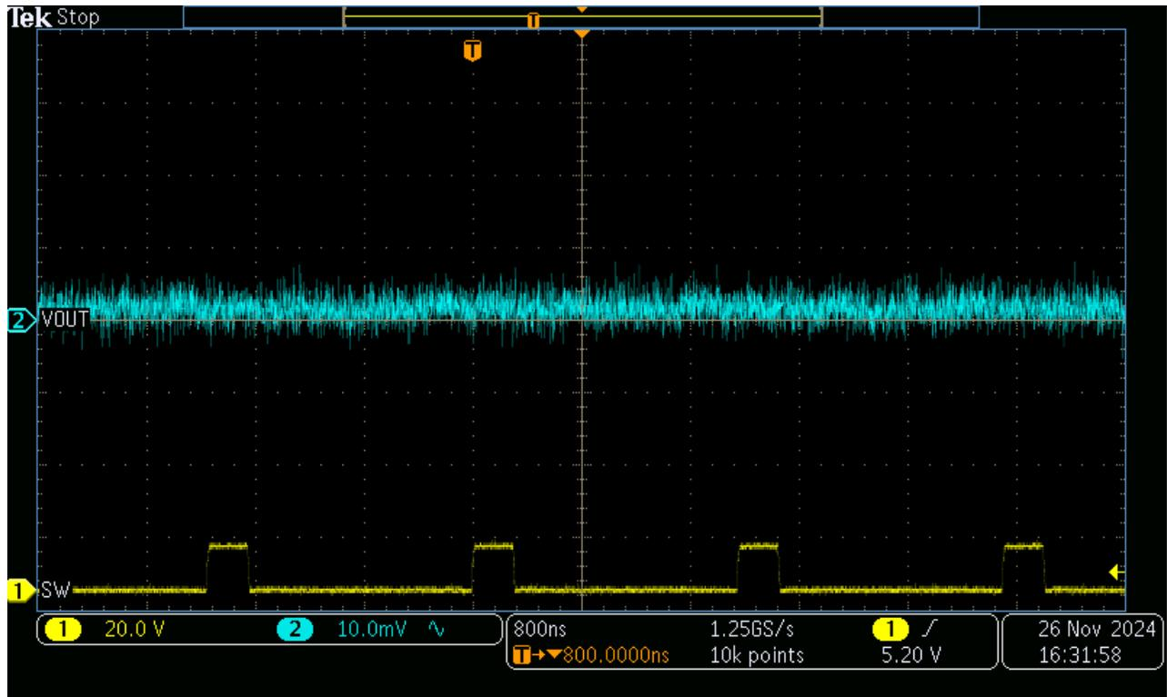
Figure 3-2. Output Voltage Ripple
