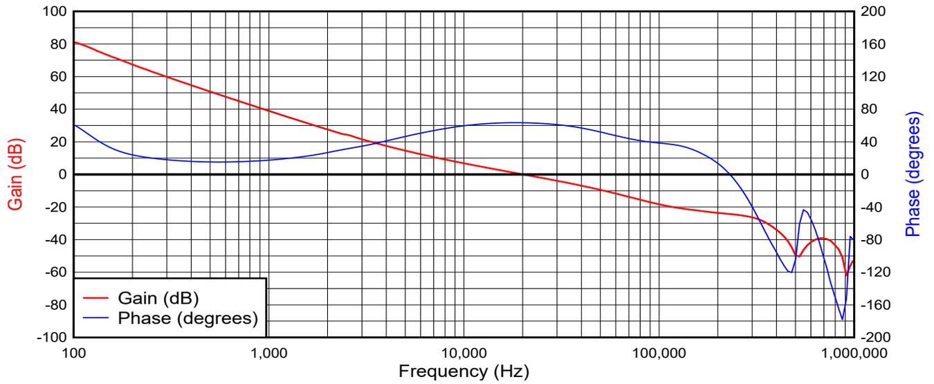
Figure 3-6. Frequency Response IOUT = 24A
