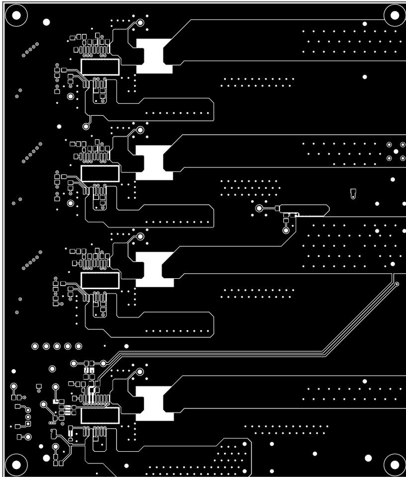
**Figure 4-7. Layer 1 (Top View)**
