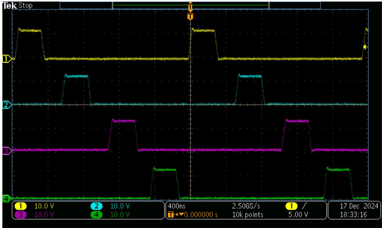
**Figure 3-1. Quadrature Switch Nodes**
