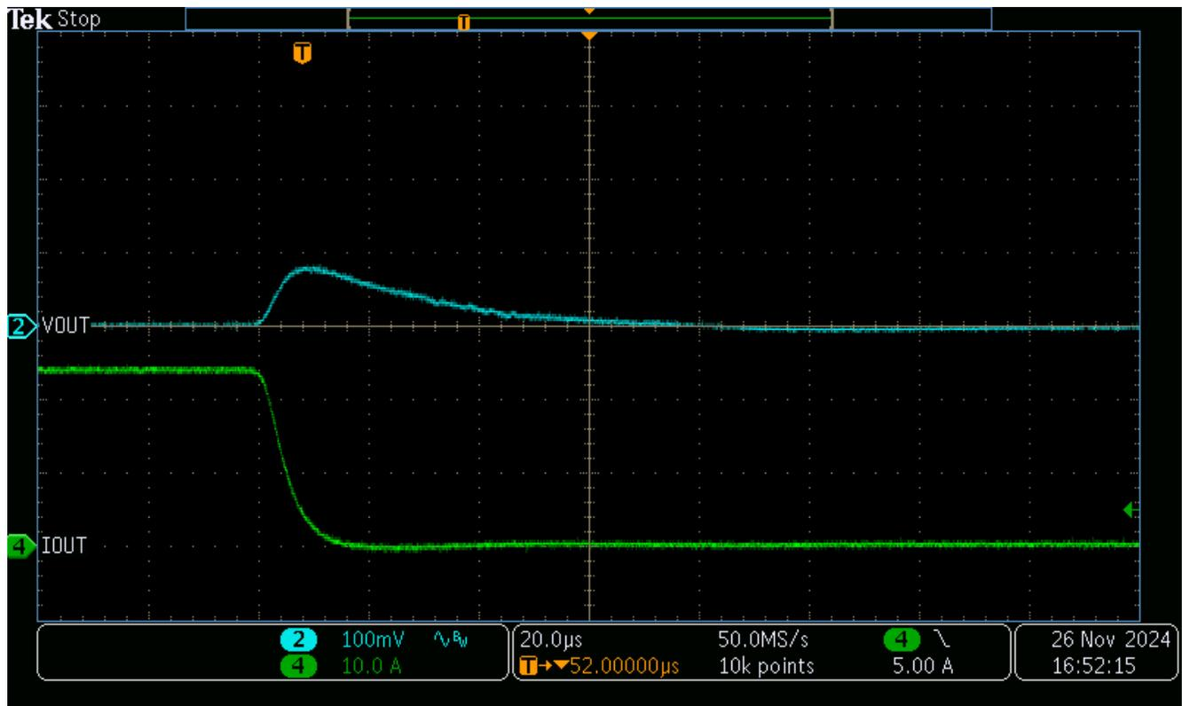
Figure 3-5. Transient Response to Load Step 24A to 500mA
