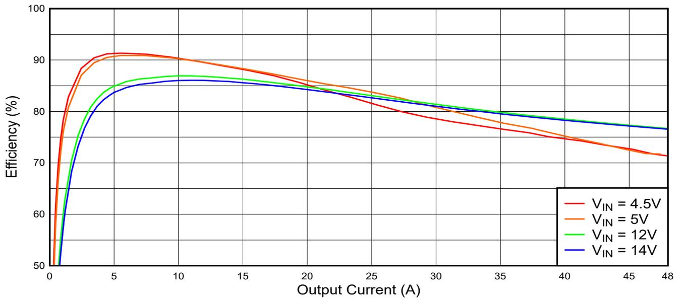
Figure 3-8. Efficiency FSW = 200kHz
