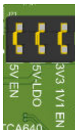
Figure 2-5. J21 Power Supply Control
