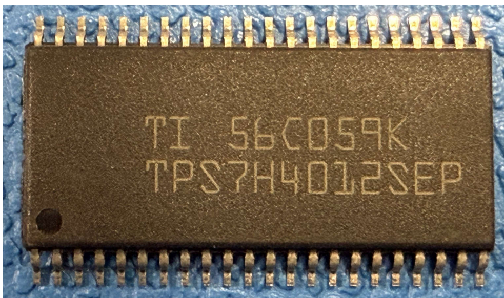
Figure 1-1. TPS7H4012-SEP Device Used in Exposure (Front)
