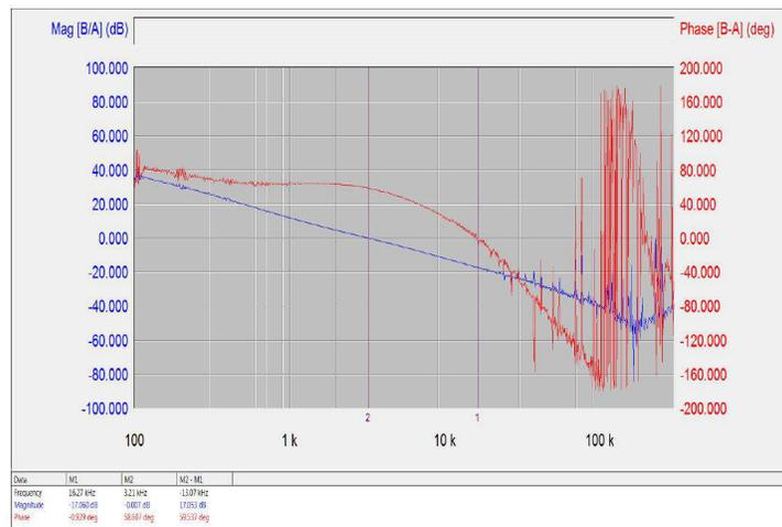
Figure 5-2. Loop Bode Plot with Amplifier
