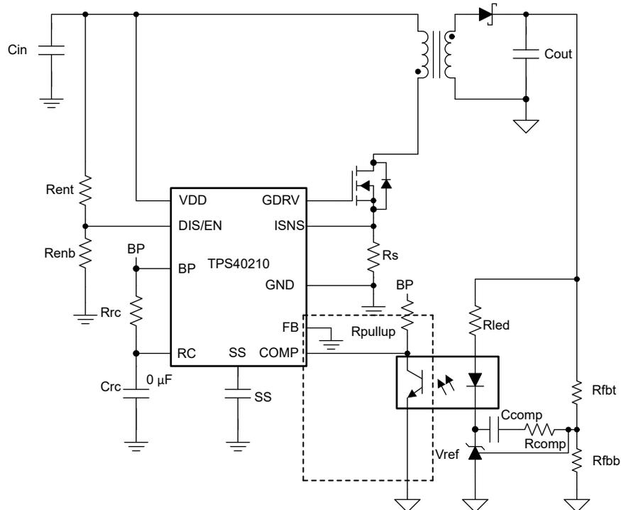
**Figure 3-1. Feedback Implementation of Secondary Side Regulation**
