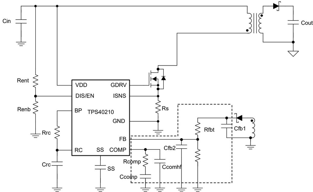
**Figure 2-1. Primary Side Regulation Block Diagram**
