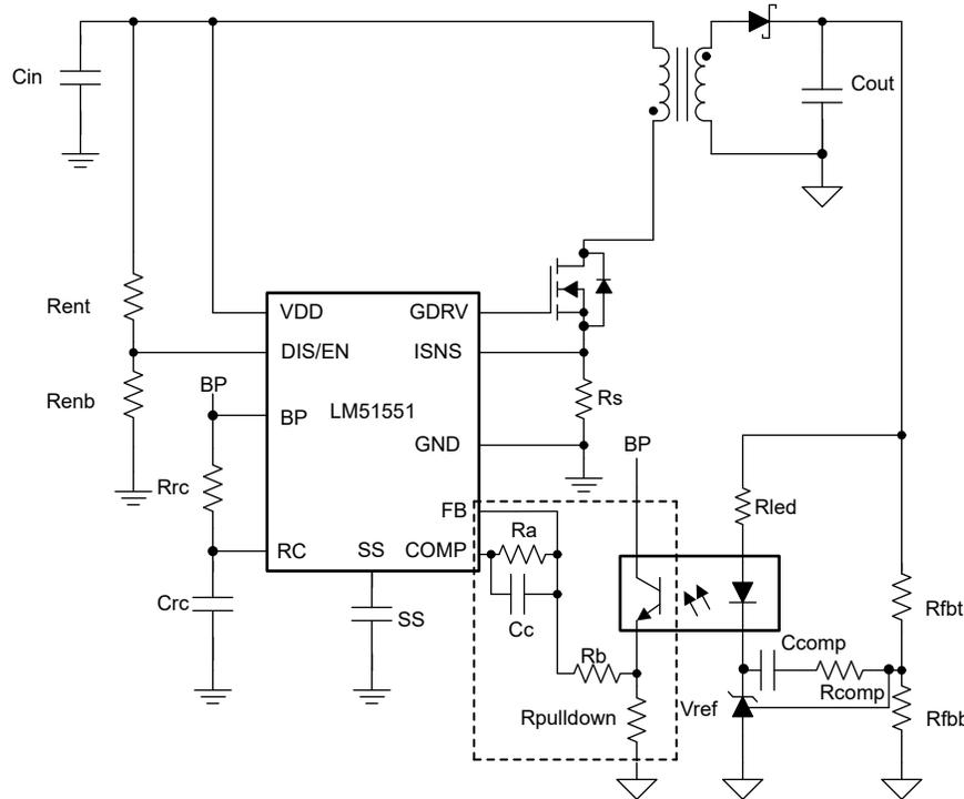
**Figure 3-2. Feedback of Secondary Side Regulation Implementation with Primary Amplifier**
