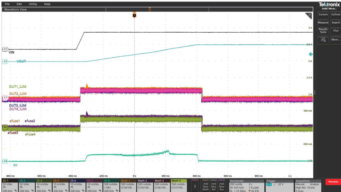
**Figure 3-6. Current Distribution Among Four TPS1685 eFuses During Start-up**
