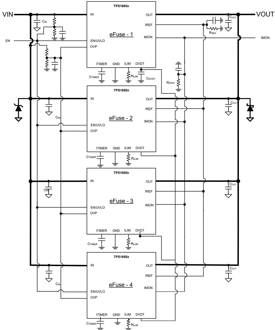
**Figure 3-4. eFuse Devices Connected in Parallel with Common Over Current Limit and ACS to Support 80A Load Current**
