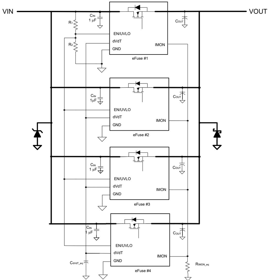
**Figure 3-2. eFuse Devices Connected in Parallel with Common Over Current Limit to Support 80A Load Current**
