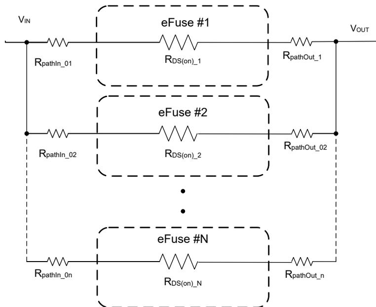
Figure 2-1. Number of  $N$  eFuse Devices Connected in Parallel Configuration
