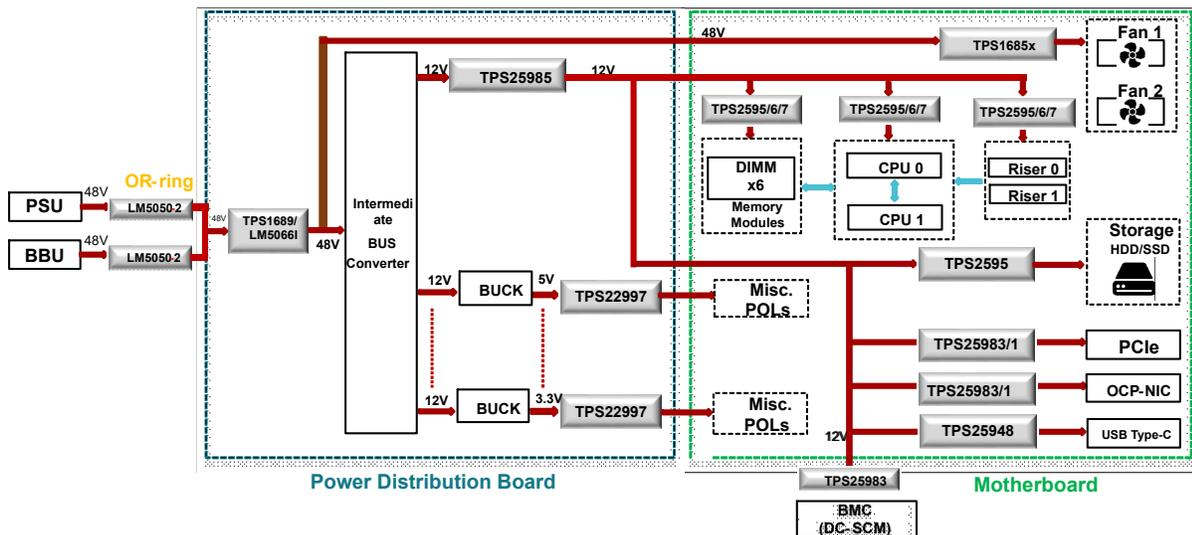
Figure 1-1. 48V Rack Server Architecture
