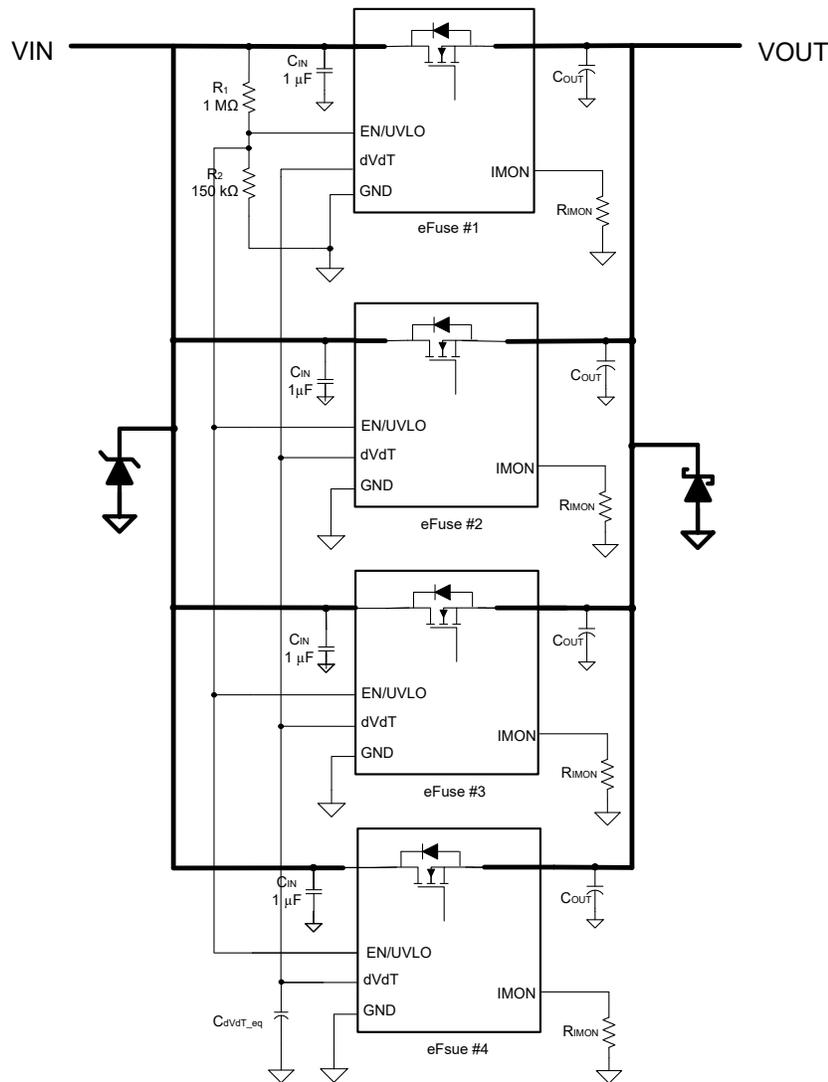
**Figure 3-1. eFuse Devices Connected in Parallel with Individual Over Current Limit to Support 80A Load Current**
