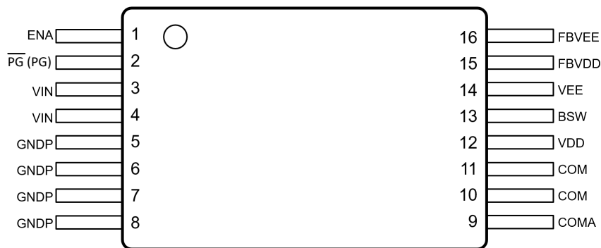
Figure 1-1. DHA Package, 16-Pin SSOP (top view)
