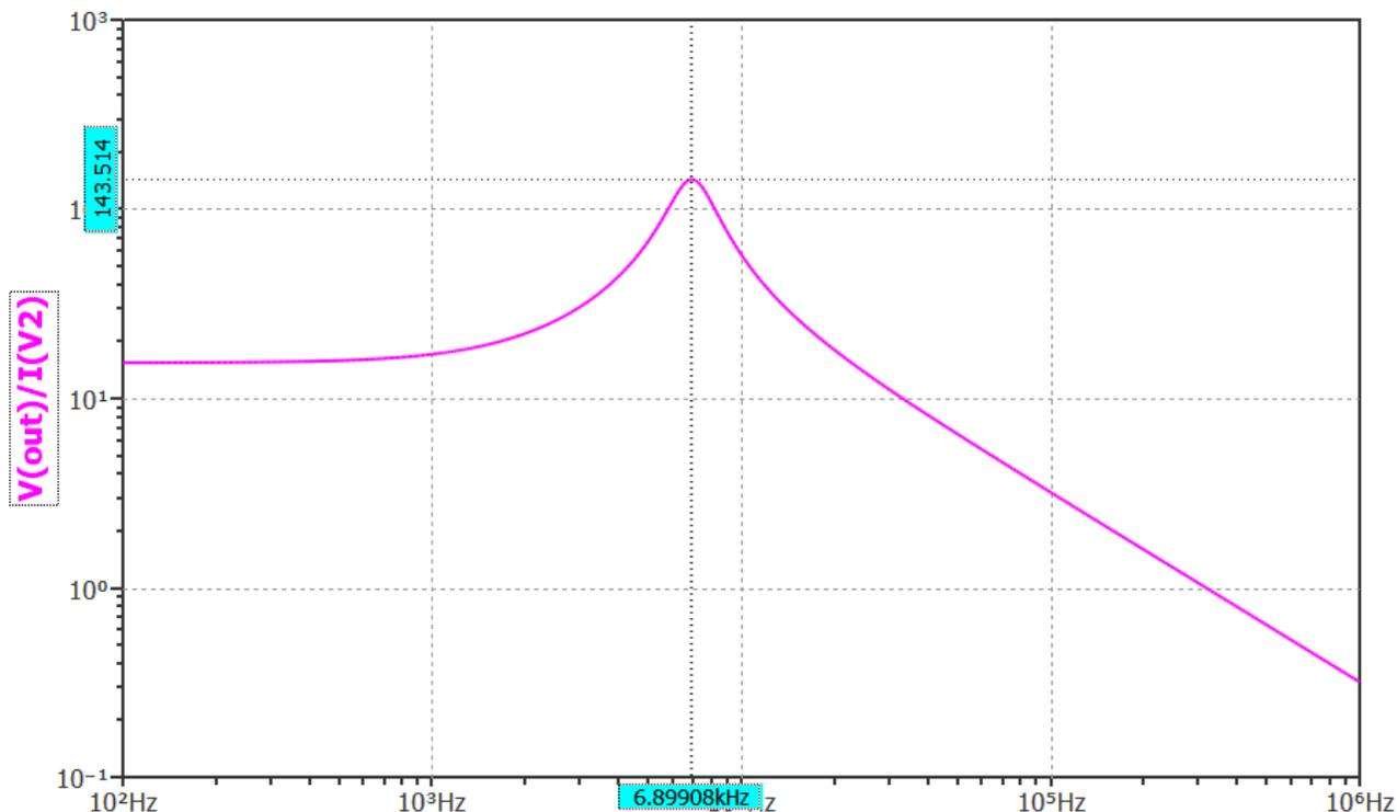
Figure 4-3. Impedance Plot for the Parallel Resonant Tank
