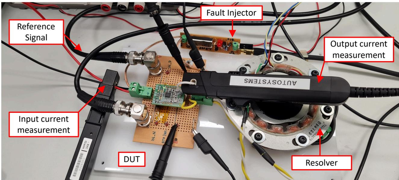
Figure 5-21. Test Setup for Fail Events
