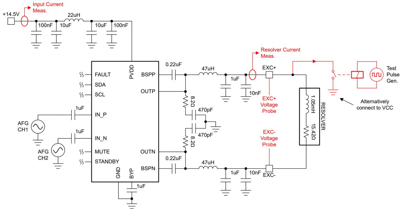
Figure 5-22. Circuit for the Test Setup for Fail Events
