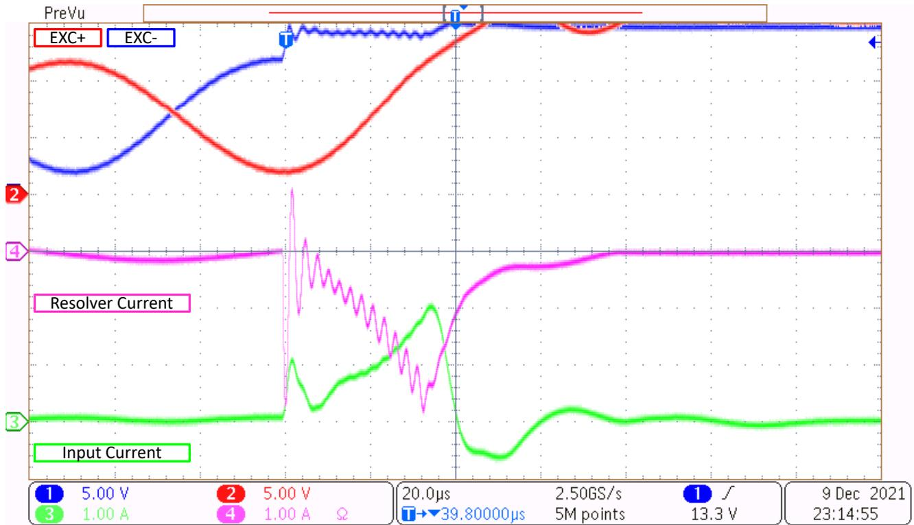
Figure 5-28. Short to VCC (Detail)
