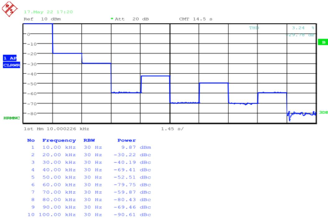
Figure 5-20. Total Harmonic Distortion (PWM signal)
