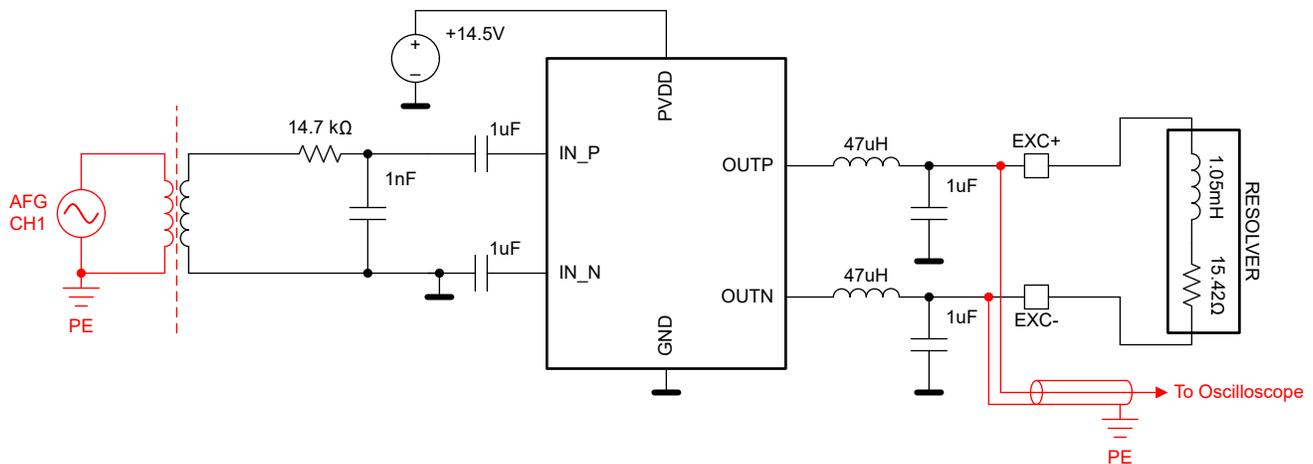
Figure 5-4. Test Setup for the Transfer Function Measurement
