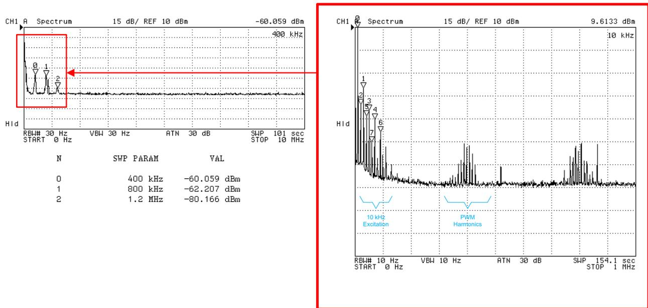
Figure 5-15. Output Spectrum of the Excitation Amplifier (Harmonic Input)
