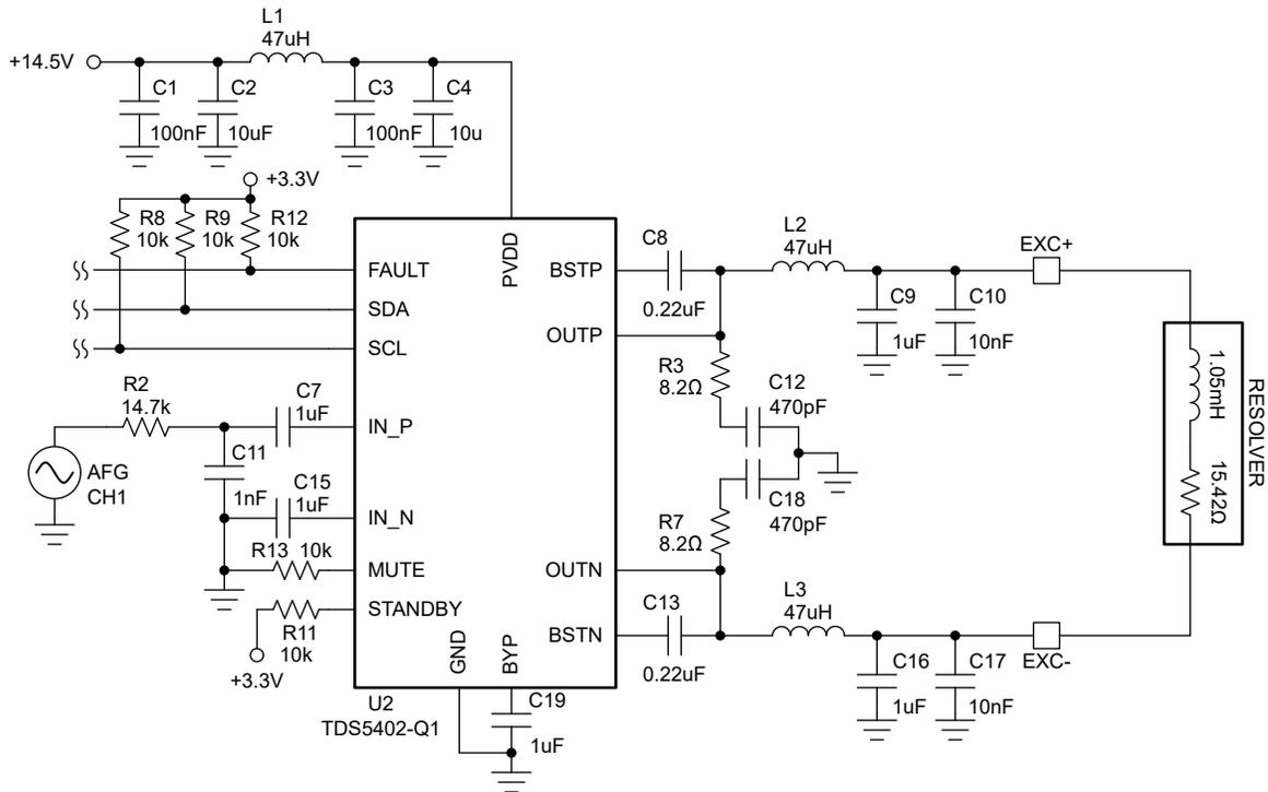
**Figure 4-1. TSD5402-Q1 Resolver Excitation Amplifier Schematic**
