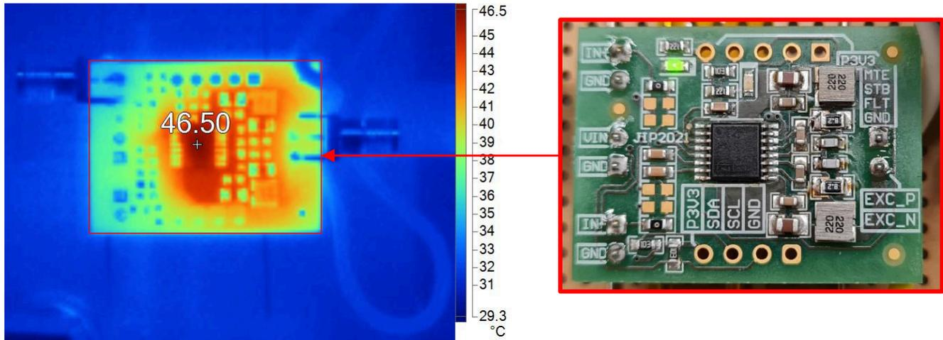
Figure 5-11. Thermal Picture of the Amplifier When Driving the Resolver
