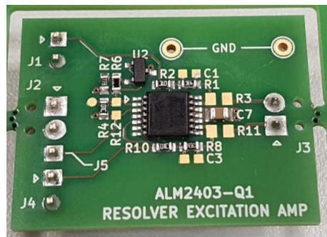
Figure 2-2. Resolver Excitation Amplifier With ALM2403-Q1 (Basic Circuit)
