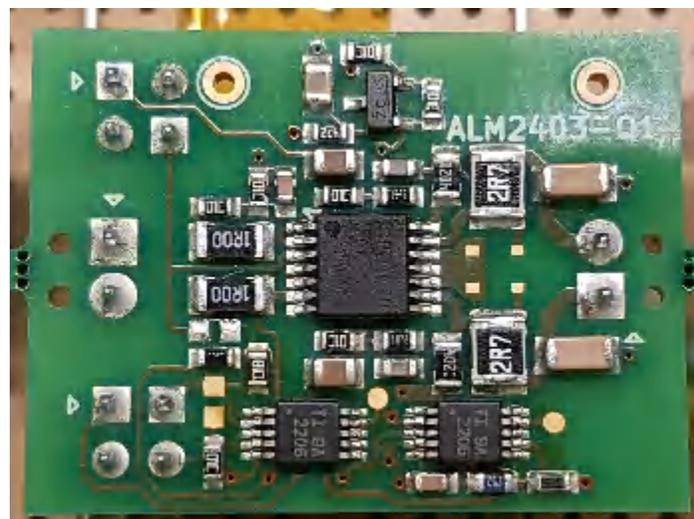
Figure 2-4. Resolver Excitation Amplifier With ALM2403-Q1 (With Advanced Overcurrent Protection)
