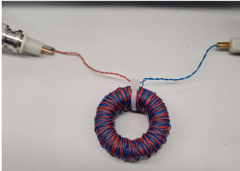
Figure 5-5. Self-Made Isolation Transformer
