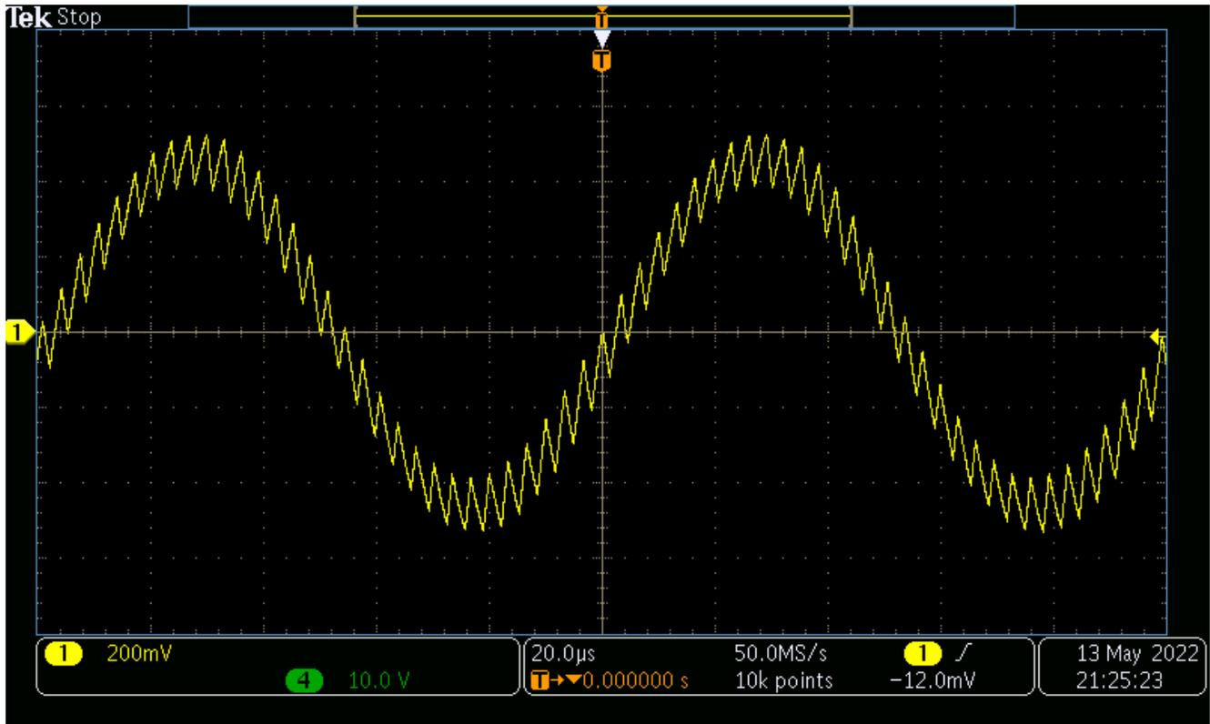
Figure 5-9. Voltage on the Input RC Filter (Across C11)
