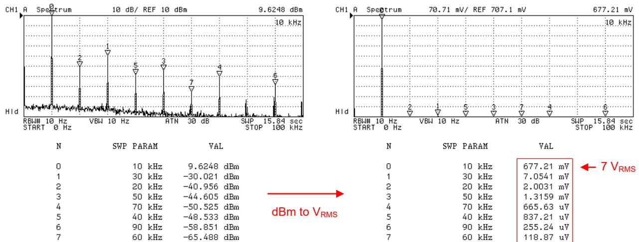
Figure 5-16. Detailed Analysis of the Output Spectrum 0-100kHz
