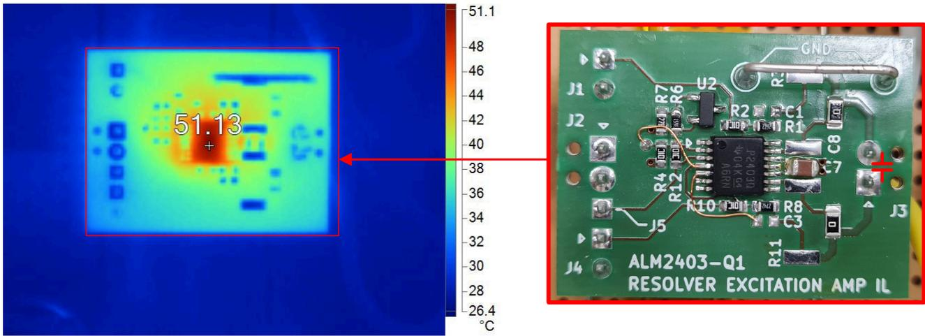
Figure 5-13. Thermal Picture of the Amplifier With Power OPAMP ALM2403-Q1 and Capacitor on the Output
