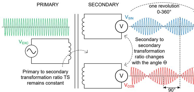
**Figure 1-4. Resolver Sensor Principle**
