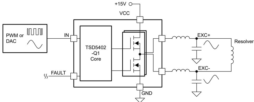
**Figure 3-1. Resolver Excitation Amplifier With Class-D Amplifier (Simplified Diagram)**
