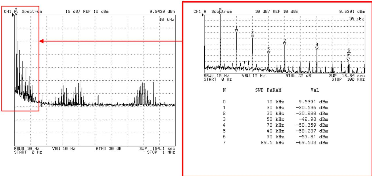
**Figure 5-18. Output Spectrum of the Excitation Amplifier (PWM Input)**
