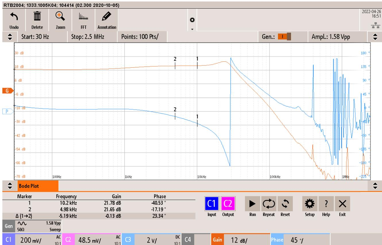
Figure 5-8. Amplifier Transfer Function (Resolver as a Load)
