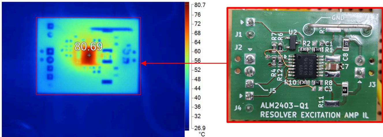
Figure 5-12. Thermal Picture of the Amplifier With Power OPAMP ALM2403-Q1
