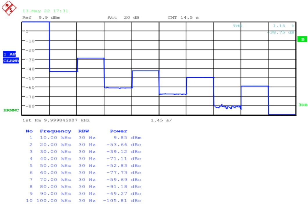
**Figure 5-19. Total Harmonic Distortion (Harmonic Signal)**
