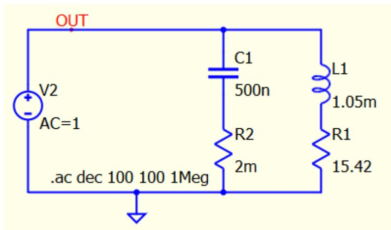
Figure 4-4. Parallel Resonant Tank Simulation Circuit (QSPICE)
