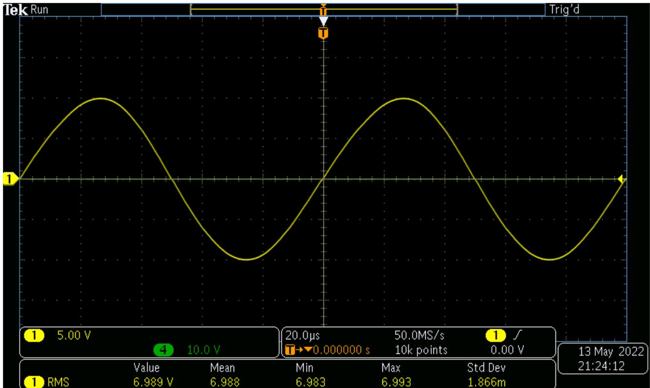
Figure 5-10. Excitation Amplifier Output Voltage
