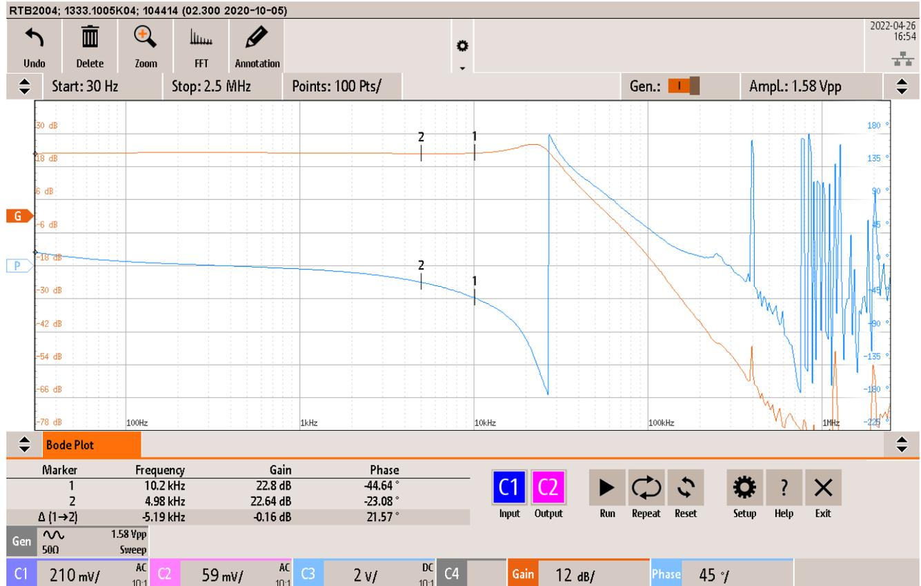
**Figure 5-7. Amplifier Transfer Function (Unloaded Output)**
