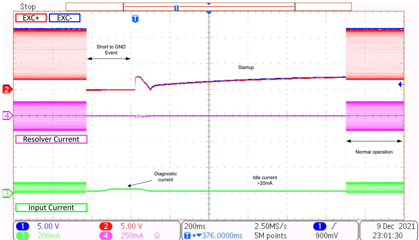
Figure 5-26. Recovery from Short to Ground
