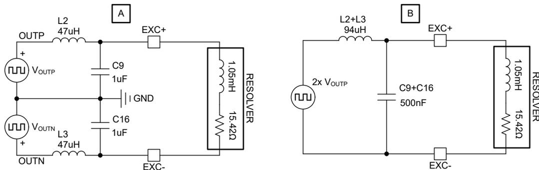
**Figure 4-2. Class-D Power Stage Analysis**
