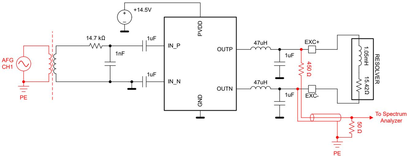
Figure 5-14. Test Setup for the Output Spectrum Measurement
