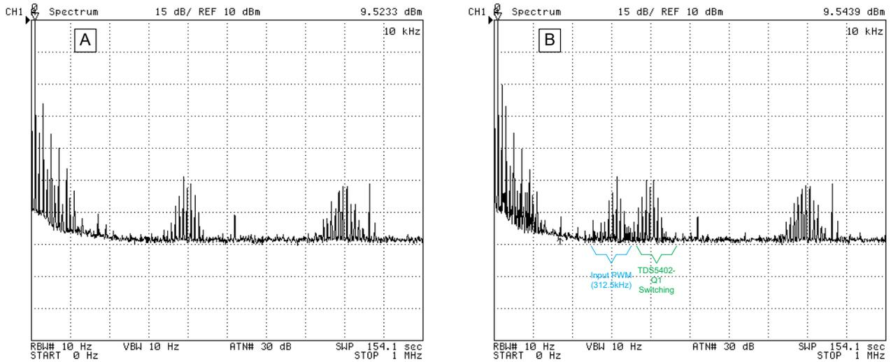
**Figure 5-17. Output Spectrum Comparison for Harmonic (A) and PWM (B) Signal Driving the Input**
