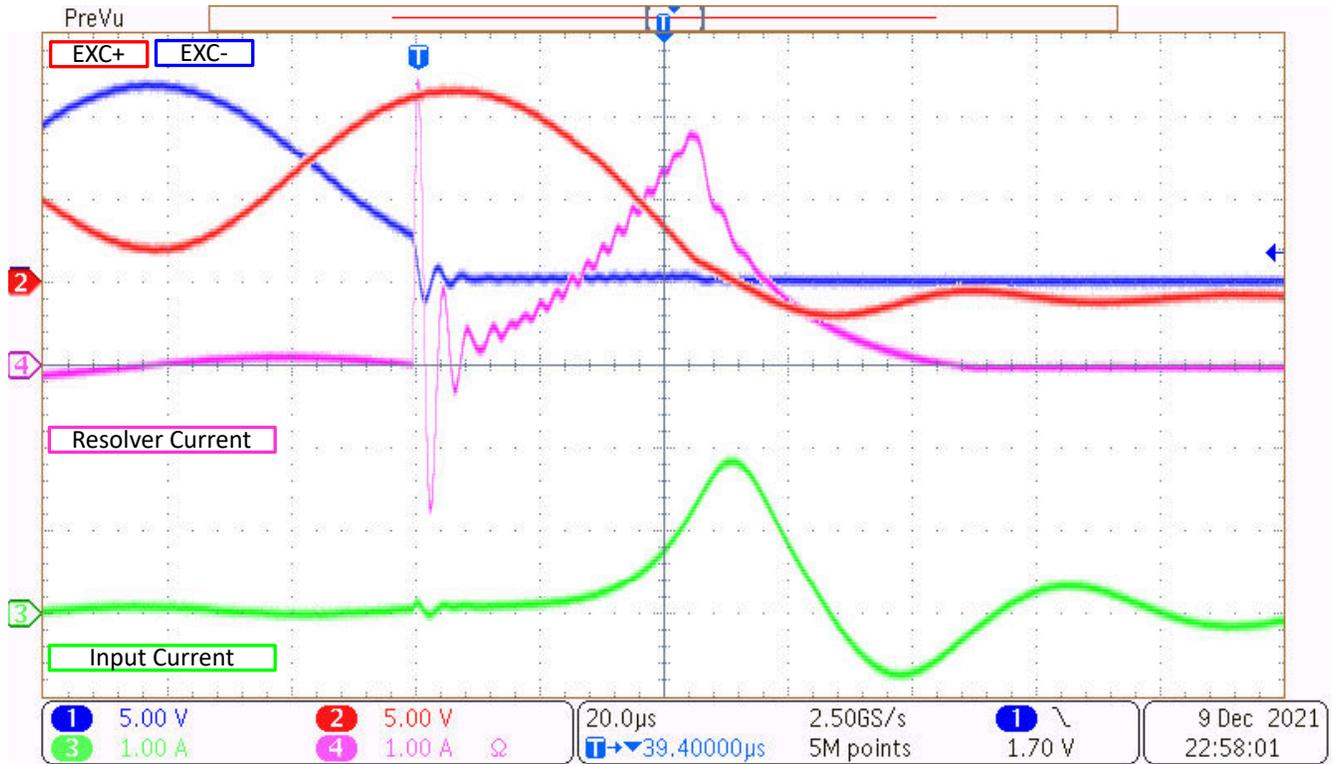
Figure 5-25. Short to Ground (detail)
