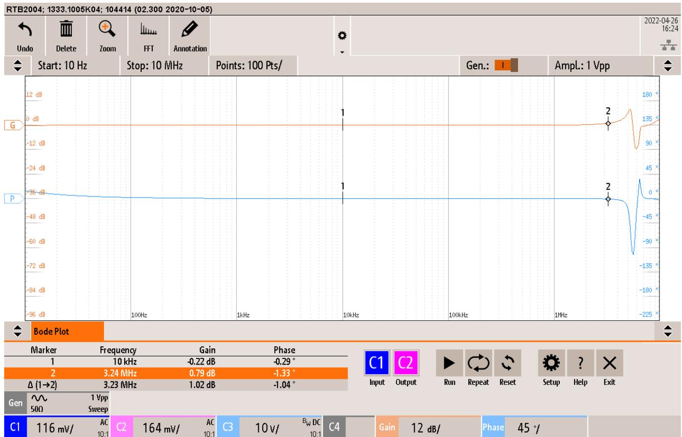
Figure 5-6. Isolation Transformer Transfer Function (High-z Loading)
