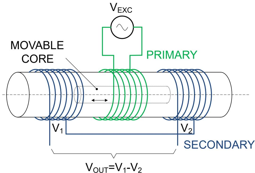
Figure 1-2. LVDT Sensor Principle
