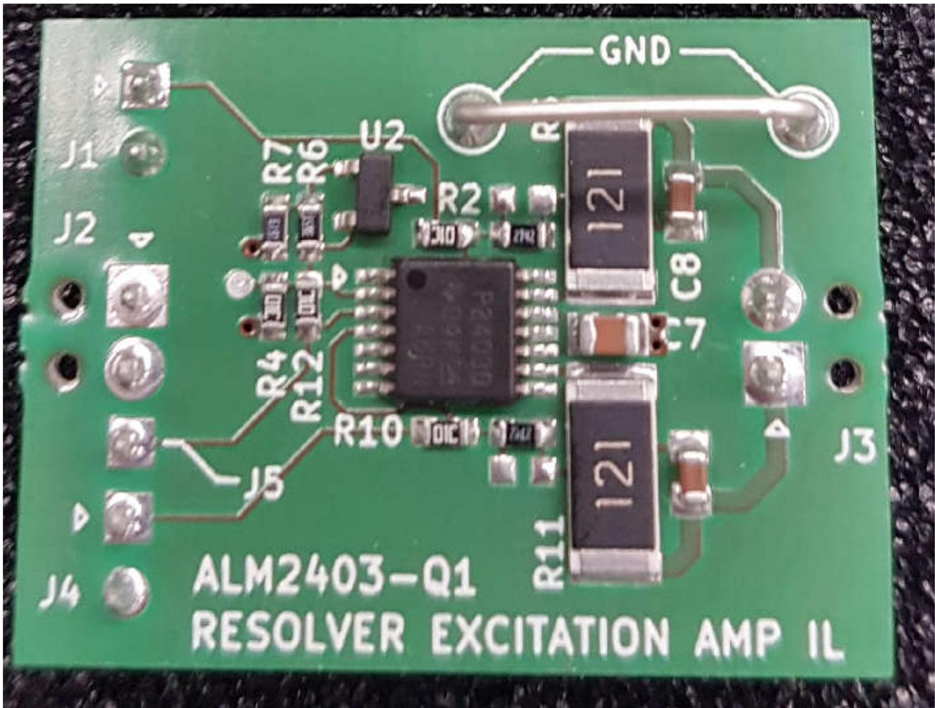
Figure 2-3. Resolver Excitation Amplifier With ALM2403-Q1 (With Output Current Limit)
