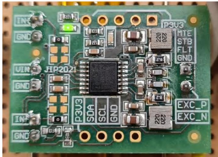
**Figure 3-2. Resolver Excitation Amplifier With TSD5402-Q1 Class-D Sensor Driver Amplifier**
