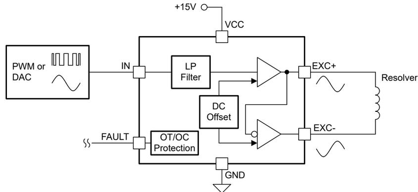
Figure 2-1. Resolver Excitation Amplifier (Simplified Diagram)
