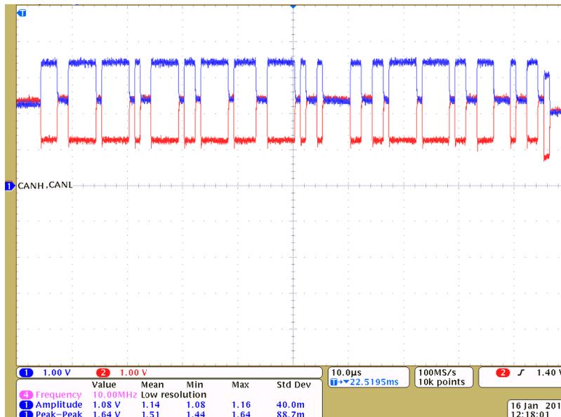
Figure 2-7. Bus Communication of a 5V SN65HVD1050 and a 3.3V SN65HVD230
