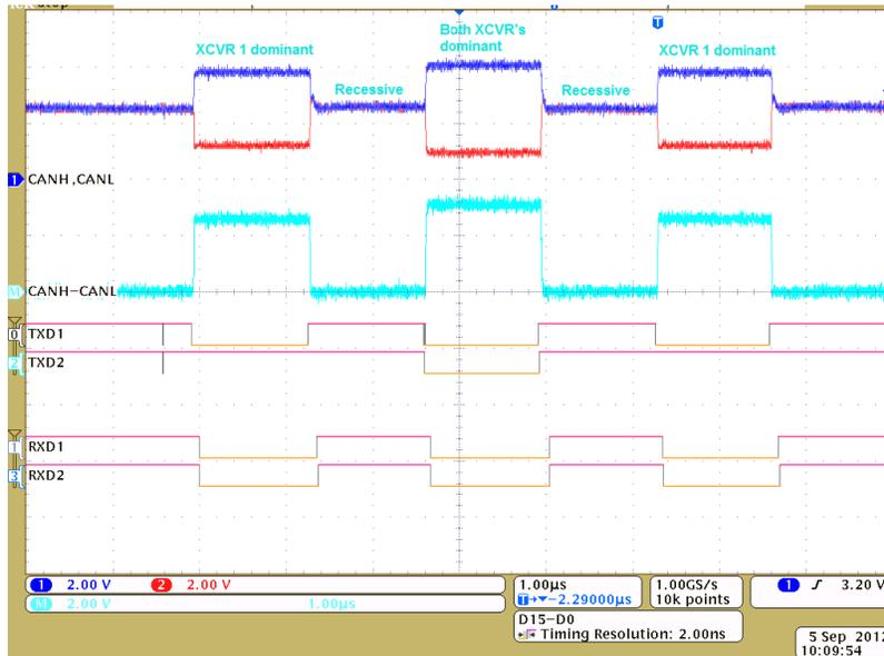
**Figure 2-1. Waveforms of Two 5V SN65HVD255 Transceivers**
