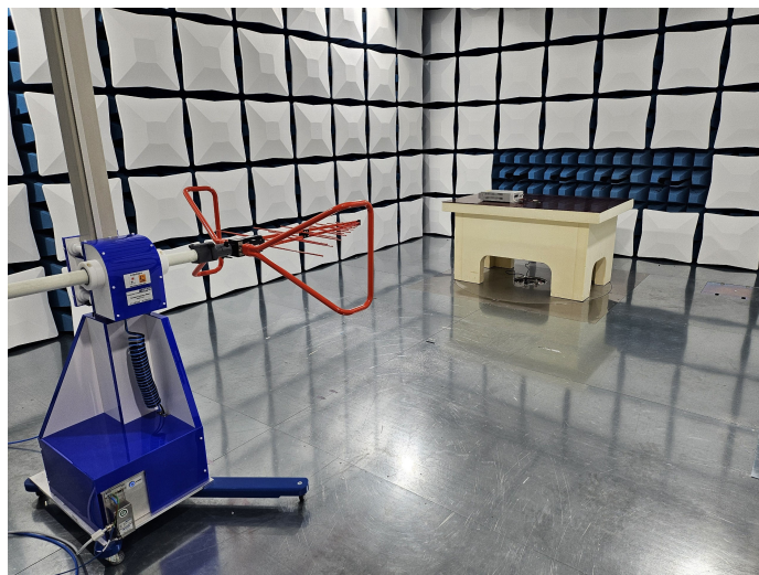
Figure 2-2. CISPR 32 RE Setup
