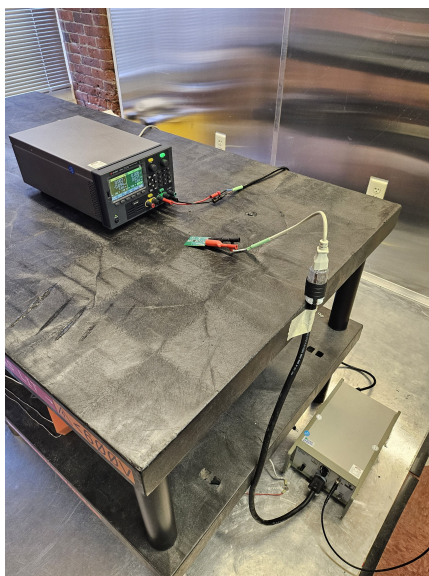
Figure 2-1. CISPR 32 CE Setup
