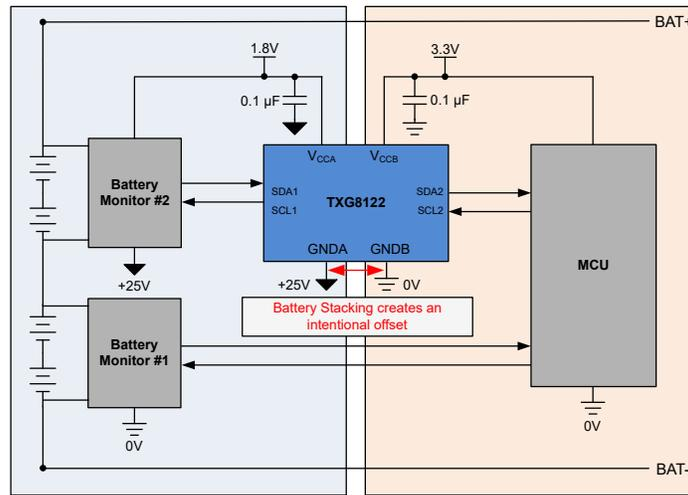
**Figure 7. Battery Stacking With TXG**
