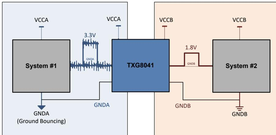
**Figure 4. AC Ground Noise**
