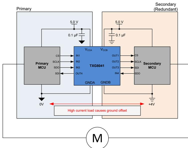
Figure 2. Electric Power Steering with TXG
