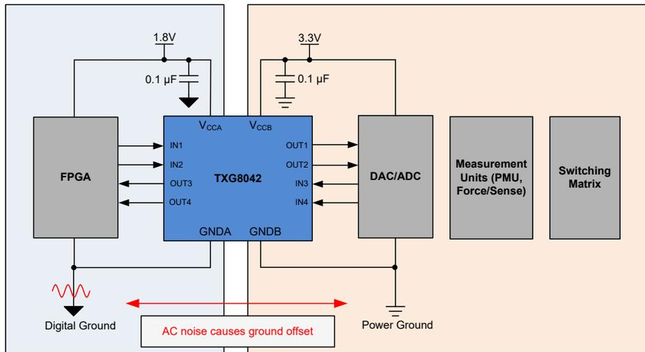
Figure 5. Semiconductor Test Equipment With TXG
