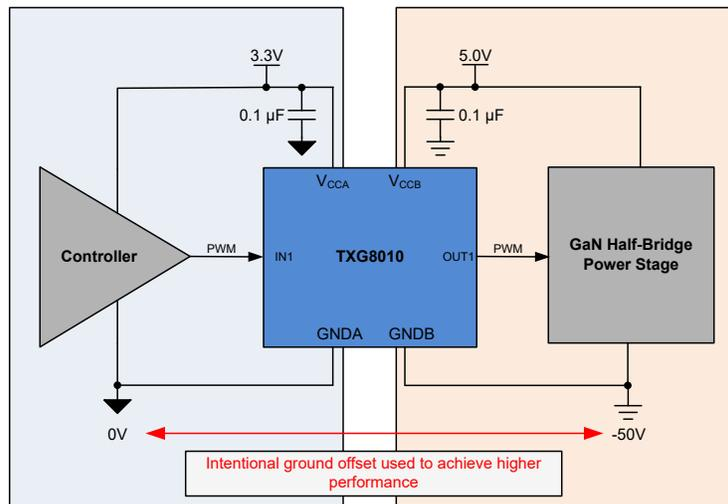
Figure 6. GaN Half-Bridge Power Stage With TXG
