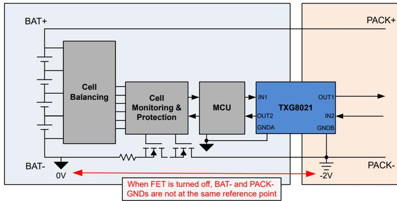
**Figure 3. Cordless Power Tool with TXG**
