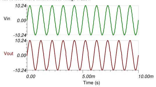
The INA828 device was simulated with a ±10.24-V differential input and a 7.75-V common-mode voltage. The following TINA simulation shows the differential input as well as the single-ended output for the INA828 device.
