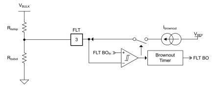
Figure 7-17. FLT Pin Brown-out Configuration Example
