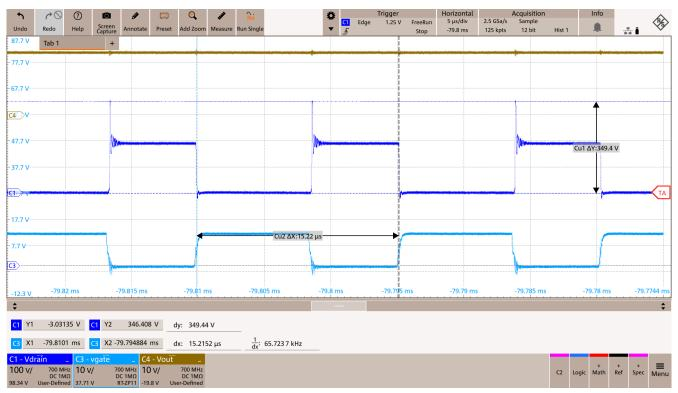
Figure 8-16. Steady State Waveform at 85Vac
