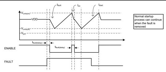
Figure 7-11. Auto-Restart Fault Diagram
