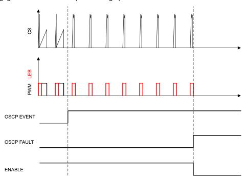
Figure 7-16. Output Short-Circuit Protection Diagram
