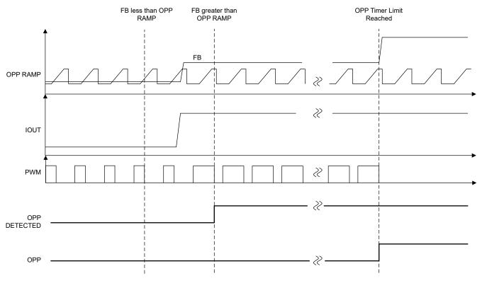
Figure 7-14. Load Step Causing OPP
