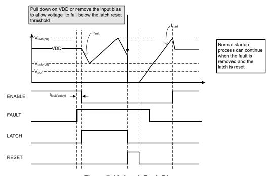
Figure 7-12. Latch Fault Diagram
