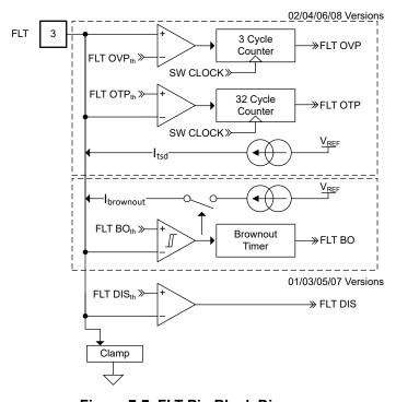
Figure 7-7. FLT Pin Block Diagram
