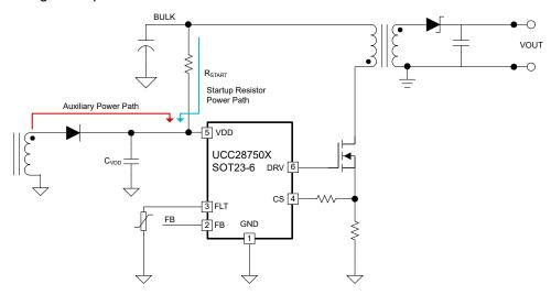
Figure 7-3. Biasing paths in a flyback application
