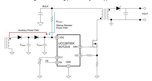
Figure 7-4. Biasing path using two diodes to split the VDD capacitance
