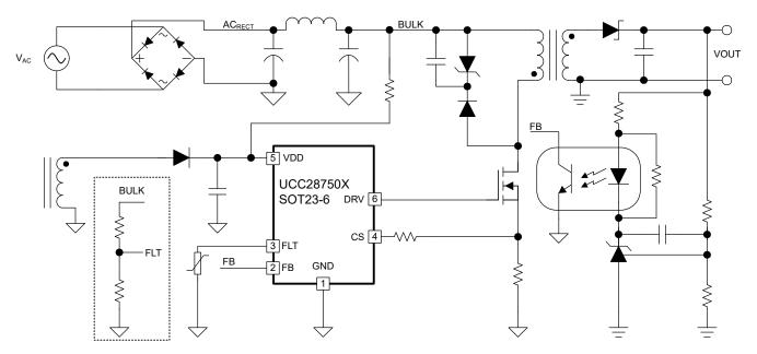
Figure 8-1. Typical Application Diagram
