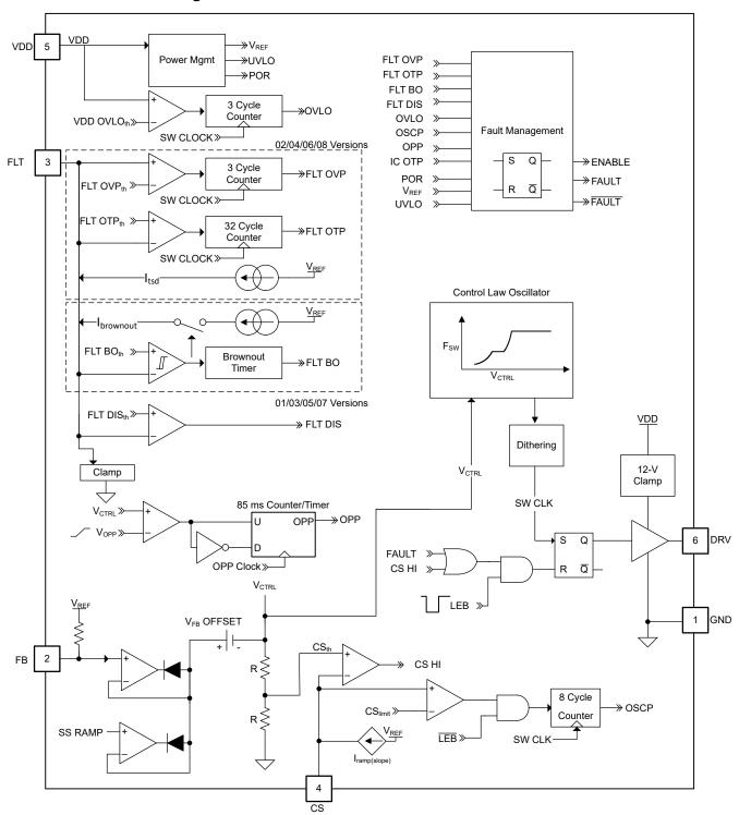
Figure 7-2. Functional Block Diagram
