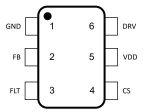
Figure 5-1. Top-view of DBV package (6 pins)
