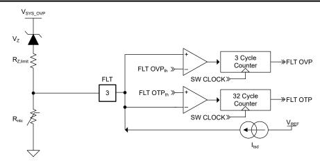
Figure 7-18. FLT Pin Overvoltage/Overtemperature Configuration Example
