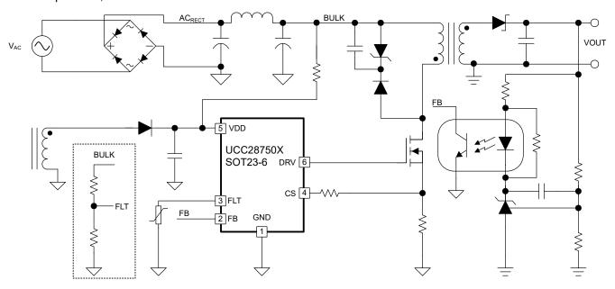
Figure 7-1. The UCC28750 in a flyback design
