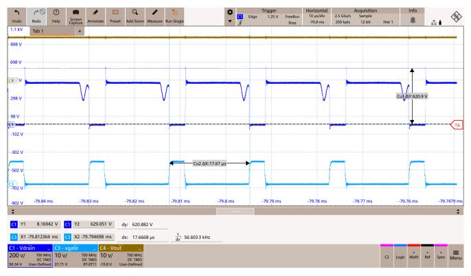
Figure 8-17. Steady State Waveform at 85Vac
