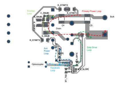
Figure 8-20. Bottom Layout of the Guidelines Schematic
