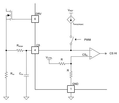
Figure 7-5. Current Sensing Pin Circuit
