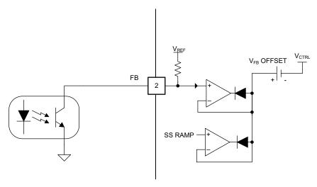
Figure 7-6. Feedback pin schematic drawing
