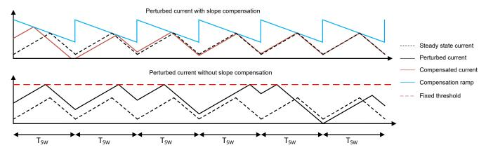
Figure 7-19. Slope Compensation in a Peak Current Mode Control Scheme
