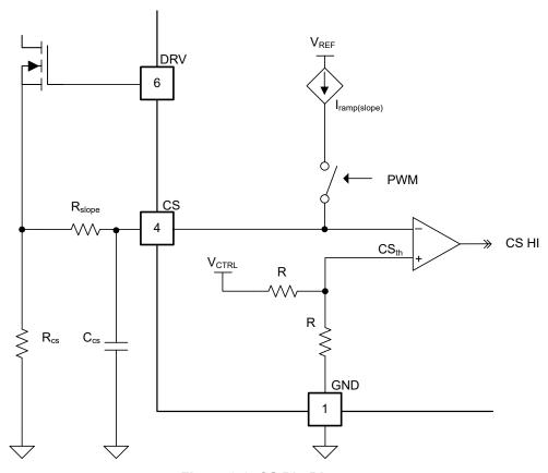
Figure 8-2. CS Pin Diagram
