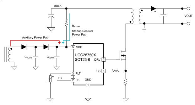
Figure 8-3. Split Diode Biasing Scheme for Use With Startup Resistors
