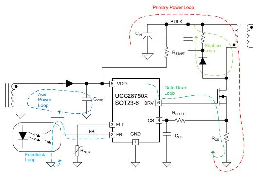
Figure 8-19. Simplified Primary Side Schematic Layout Guidelines
