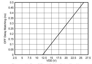
Figure 5-23. Turn-Off and Falling Delay Matching
