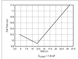
Figure 5-15. Output Fall Time vs VDD
