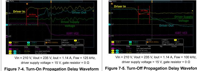
Figure 7-5. Turn-Off Propagation Delay Waveform
