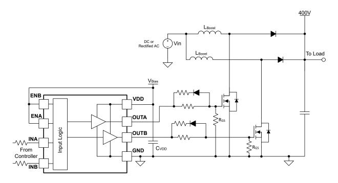
Figure 7-1. UCC27624-Q1 Typical Application Diagram
