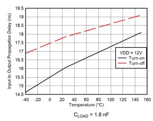
Figure 5-19. Input Propagation Delay vs Temperature
