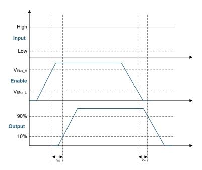
Figure 5-1. Enable Function
