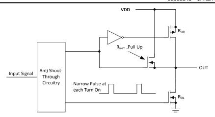
Figure 6-1. UCC27624-Q1 Gate Driver Output Structure
