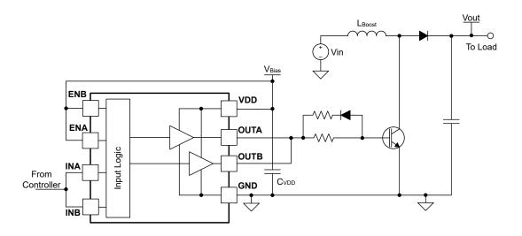
Figure 7-3. UCC27624-Q1 Used to Drive IGBT in the Boost Converter
