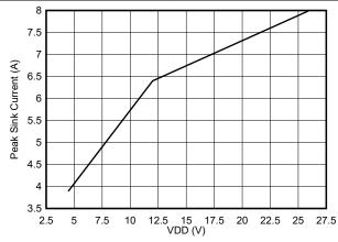
Figure 5-25. Peak Sink Current vs VDD
