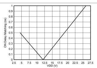
Figure 5-22. Turn-on/Rising Delay Matching
