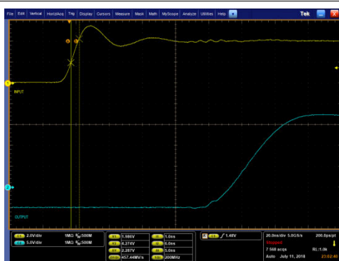
Figure 8-12. PWM Input (yellow) and Driver Output (blue) Rising Edge
