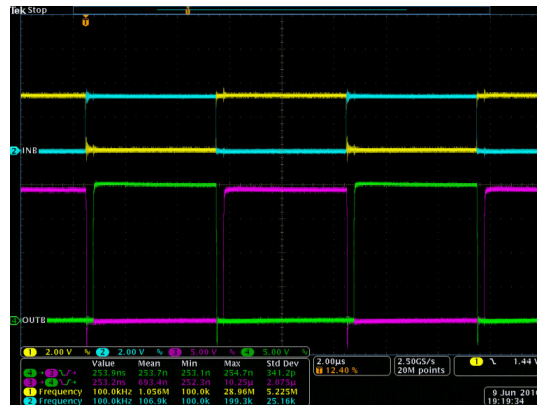
Figure 8-5. Bench Test Waveform for INA/B and OUTA/B
