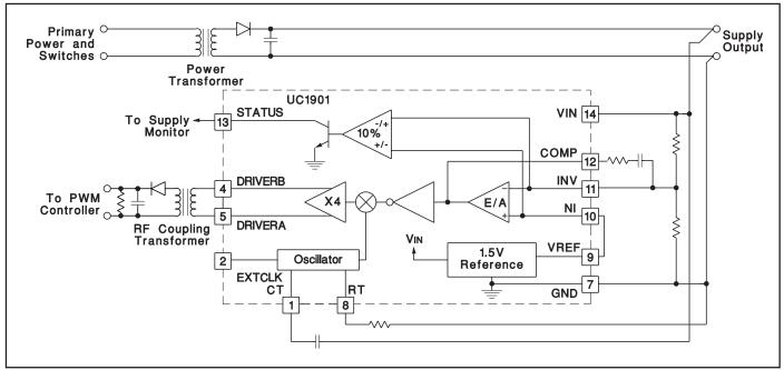
Figure 4. R.F. Transformer Coupled Feedback
