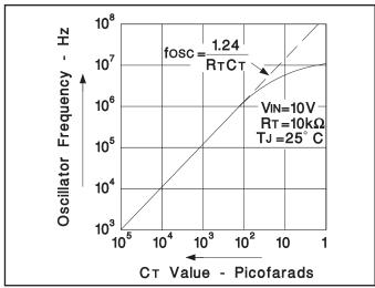
Figure 2. Oscillator Frequency
