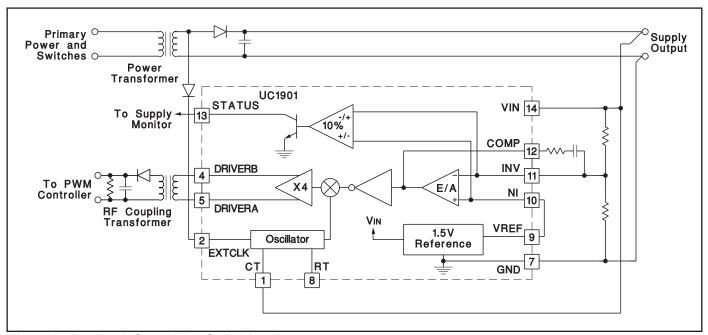
Figure 5. Feedback Coupled at Switching Frequency
