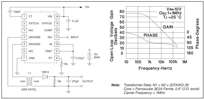
Figure 1. Transformer Coupled Open Loop Transfer Function
