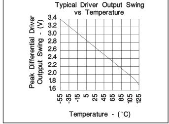
Figure 3. Typical Driver Output Swing vs Temperature
