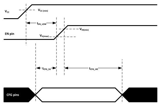
Figure 6-1. Power-On Timing Requirements
