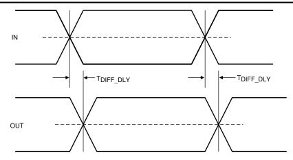
Figure 6-3. USB Propagation Delay
