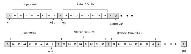
Figure 7-4. I2C Read with Repeated Start
