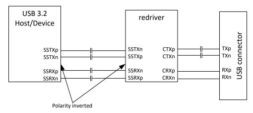
Figure 7-1. Polarity Inversion Example
