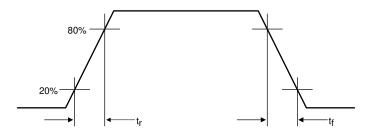
Figure 6-5. Output Rise and Fall Times
