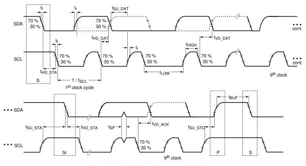
Figure 6-2. I2C Timing Diagram Definitions
