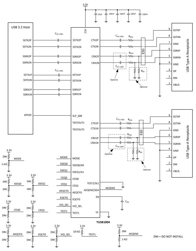
Figure 8-2. Application Circuit
