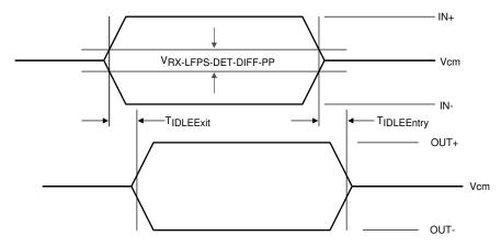
Figure 6-4. Electrical Idle Exit and Entry Delay
