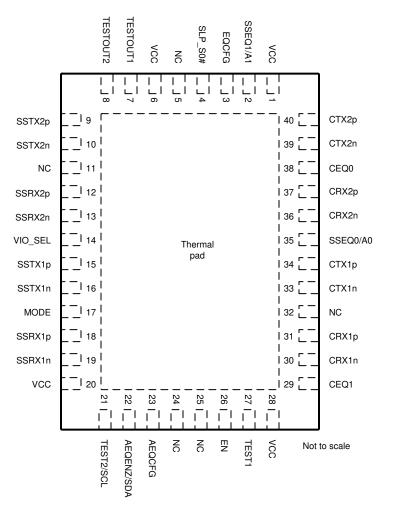
Figure 4-1. TUSB1004 RNQ Package, 40-Pin WQFN (Top View)
