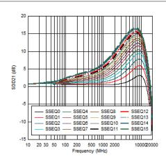
Figure 5-2. USB SSTX1 EQ Settings Curves at 85  $\Omega$  (from simulation)
