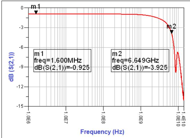
Figure 1. Differential S21 vs Frequency for Port A
