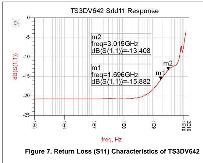
Figure 7. Return Loss (S11) Characteristics of TS3DV642
