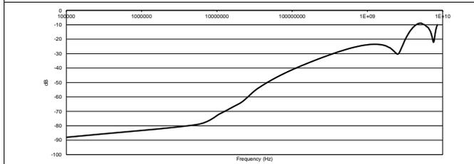
Figure 5. Off-State Isolation (OISO) for Port A
