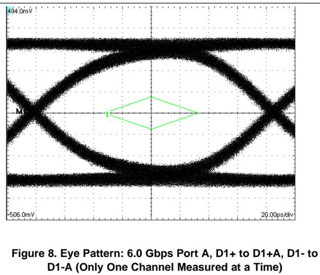
Figure 8. Eye Pattern: 6.0 Gbps Port A, D1+ to D1+A, D1- to D1-A (Only One Channel Measured at a Time)
