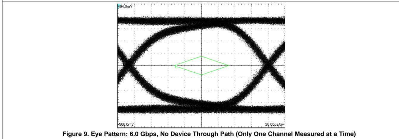
Figure 9. Eye Pattern: 6.0 Gbps, No Device Through Path (Only One Channel Measured at a Time)
