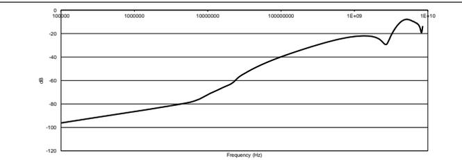
Figure 6. Off-State Isolation (OISO) for Port B
