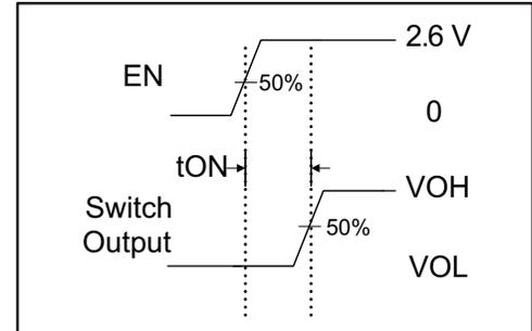
Figure 14. Switch Turn-On Time ( $t_{ON}$ )
