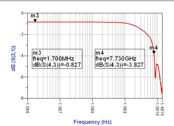
Figure 2. Differential S21 vs Frequency for Port B
