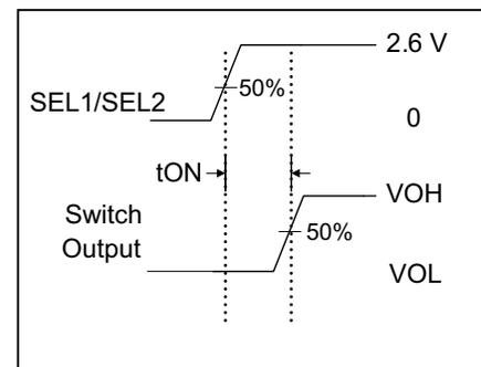
Figure 15. Switching Time Between Channels ( $t_{SWITCH}$ )
