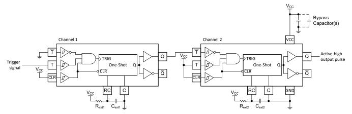
Figure 8-4. Delayed Pulse Generation Schematic Using the TPUL2T323-Q1
