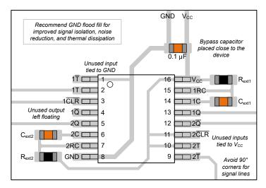
Figure 8-6. Layout Example for TPUL2T323-Q1 in the PW (TSSOP) package
