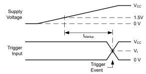
Figure 6-8. Voltage Waveforms, Startup Time
