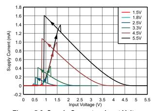
Figure 5-3. Supply Current vs Input Voltage
