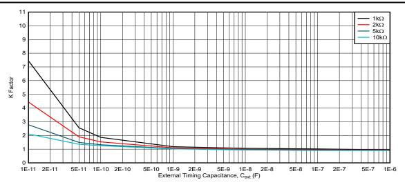
Figure 5-12. K Factor,  $V_{CC}$  = 2.5V,  $R_{ext}$  = 1k $\Omega$  to 10k $\Omega$
