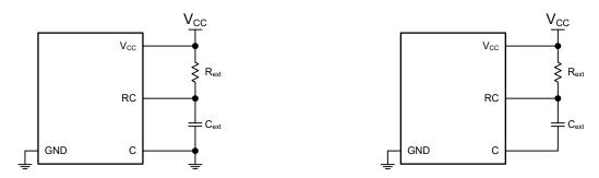
Figure 7-1. Timing component connection, with and without external ground
