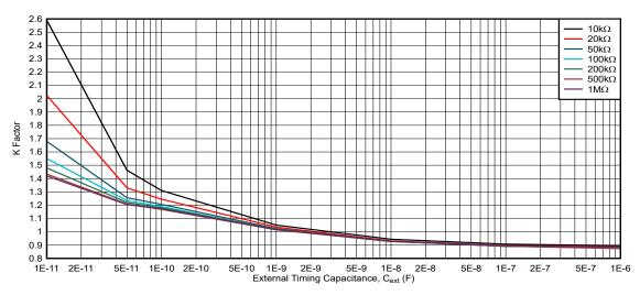
Figure 5-11. K Factor,  $V_{CC}$  = 1.8V,  $R_{ext}$  = 10k $\Omega$  to 1M $\Omega$
