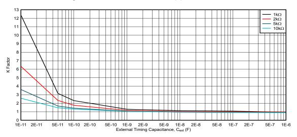
Figure 5-10. K Factor,  $V_{CC}$  = 1.8V,  $R_{ext}$  = 1k $\Omega$  to 10k $\Omega$
