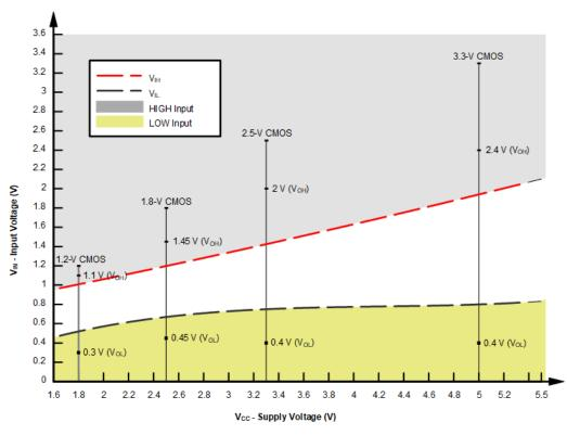
Figure 7-4. TPULxT Input Voltage Levels
