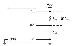
Figure 8-2. External protection diode connection
