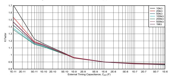
Figure 5-19. K Factor,  $V_{CC}$  = 5.5V,  $R_{ext}$  = 10k $\Omega$  to 1M $\Omega$
