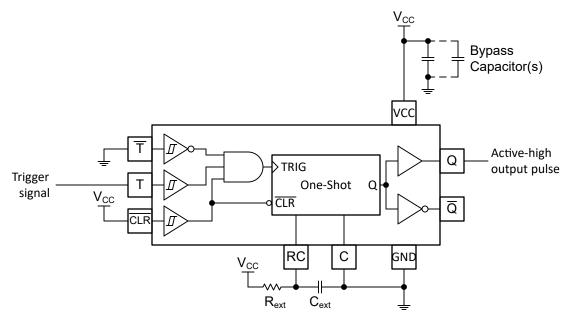
Figure 8-1. Pulse Generator Schematic Using the TPUL2T323-Q1
