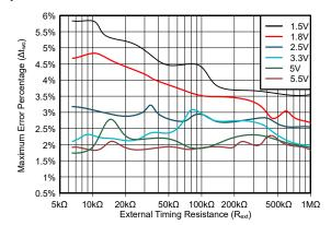
Figure 5-24. Maximum output pulse width error (absolute value) versus timing resistor values with C<sub>ext</sub> = 1nF
