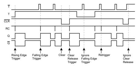
Figure 5-1. Input/Output Timing Diagram
