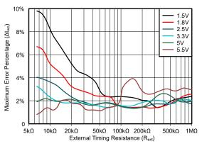
Figure 5-23. Maximum output pulse width error (absolute value) versus timing resistor values with  $C_{\text{ext}} = 100 \text{pF}$
