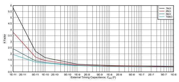
Figure 5-14. K Factor,  $V_{CC}$  = 3.3V,  $R_{ext}$  = 1k $\Omega$  to 10k $\Omega$
