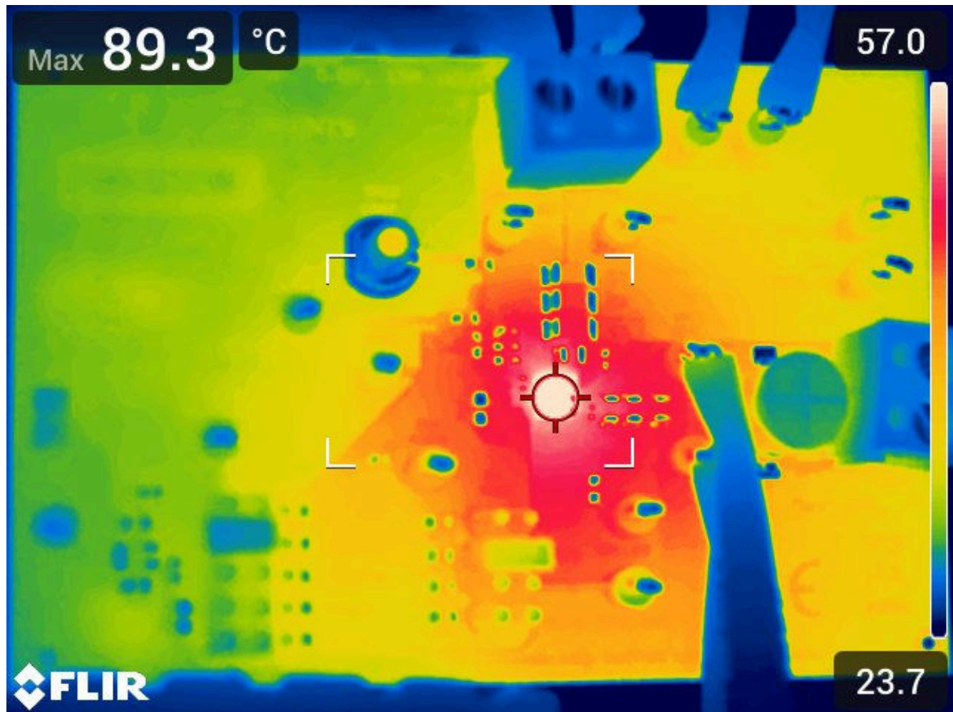
Figure 7-20. Thermal Image at 25^{\circ}\text{C} Ambient
