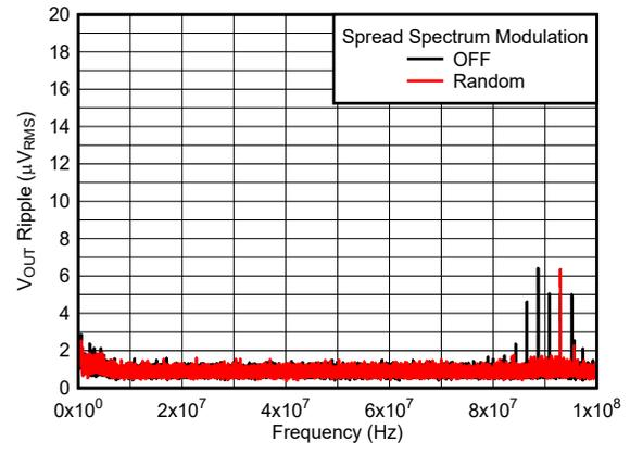
5 V to 1.2 V, 1 A 2.2  $\mu\text{H}$ , 2.2 MHz First and second L-C
