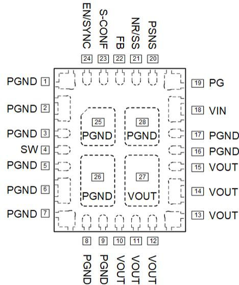
**Figure 5-1. 28-Pin QFN RDU Package (Top View)**
