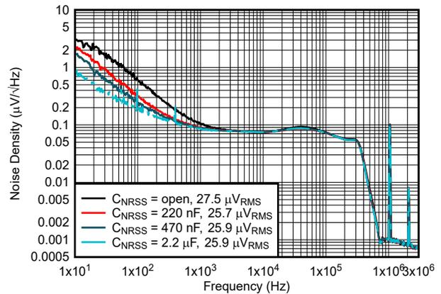
12 V to 1.8 V    1 MHz    After ferrite bead filter
