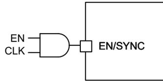
**Figure 7-1. Synchronization with Separate Enable Signal (Optional)**
