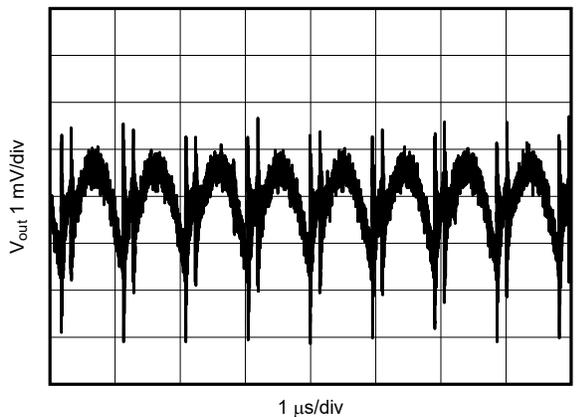
12 V to 1.8 V, 1 A    2.2  $\mu\text{H}$ , 1 MHz    First L-C Only
