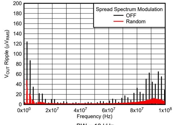
5 V to 1.2 V, 1 A 2.2  $\mu\text{H}$ , 2.2 MHz First L-C Only
