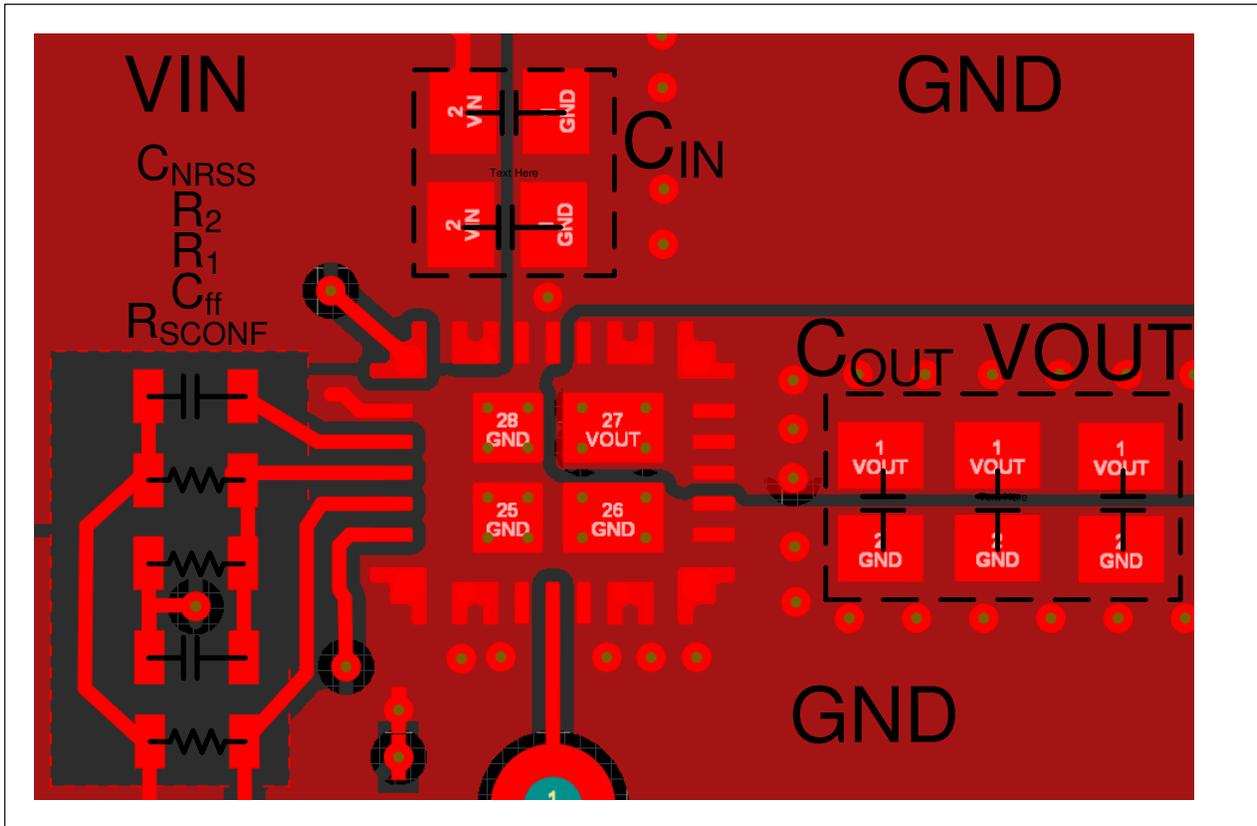
Figure 8-15. Recommended Layout for Single L-C Filter
