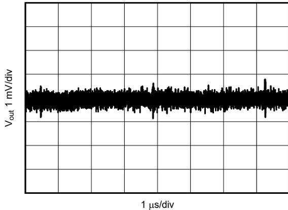
5 V to 1.8 V, 1 A 2.2  $\mu\text{H}$ , 2.2 MHz First and second L-C
