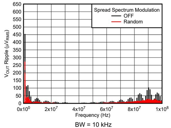
12 V to 1.8 V, 1 A    2.2  $\mu\text{H}$ , 1 MHz    First L-C Only
