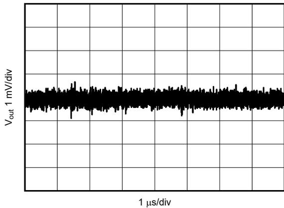
5 V to 1.2 V, 1 A 2.2  $\mu\text{H}$ , 2.2 MHz First and second L-C
