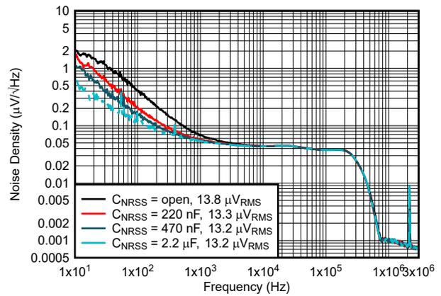
5 V to 1.2 V    2.2 MHz    After ferrite bead filter
