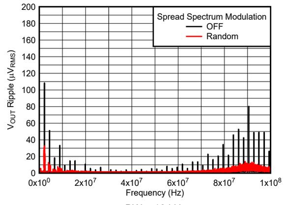
5 V to 1.8 V, 1 A 2.2  $\mu\text{H}$ , 2.2 MHz First L-C Only
