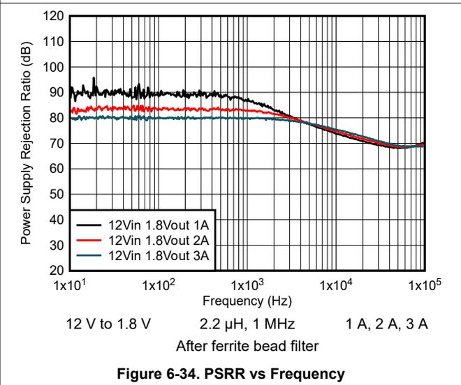
**Figure 6-34. PSRR vs Frequency**
