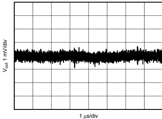
12 V to 1.8 V, 1 A 2.2  $\mu\text{H}$ , 1 MHz First and second L-C
