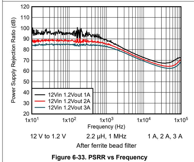
**Figure 6-33. PSRR vs Frequency**
