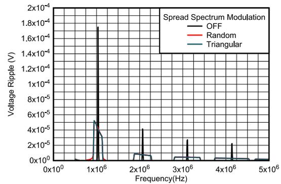
12 V to 1.2 V, 2 A    2.2  $\mu\text{H}$ , 1 MHz    BW = 10 kHz
