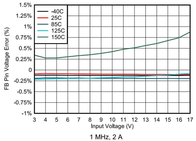
**Figure 6-38. FB Pin Voltage Error vs Input Voltage**
