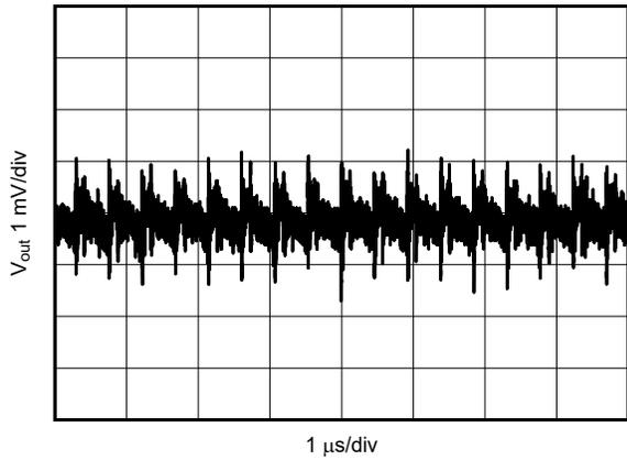
5 V to 1.2 V, 1 A 2.2  $\mu\text{H}$ , 2.2 MHz First L-C Only
