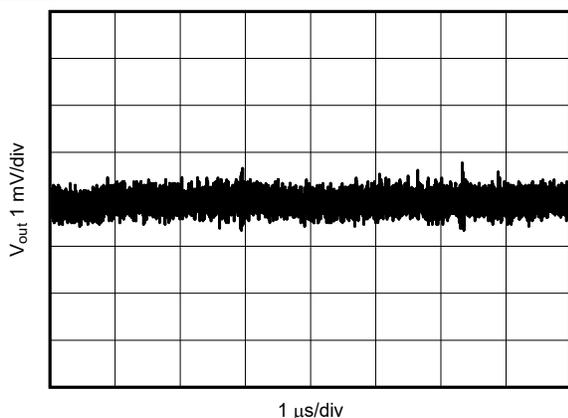
5 V to 3.3 V, 1 A 2.2  $\mu\text{H}$ , 2.2 MHz First and second L-C
