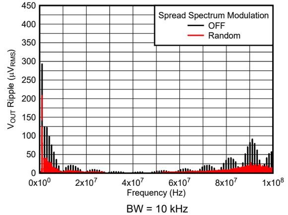
12 V to 1.2 V, 1 A    2.2  $\mu\text{H}$ , 1 MHz    First L-C Only
