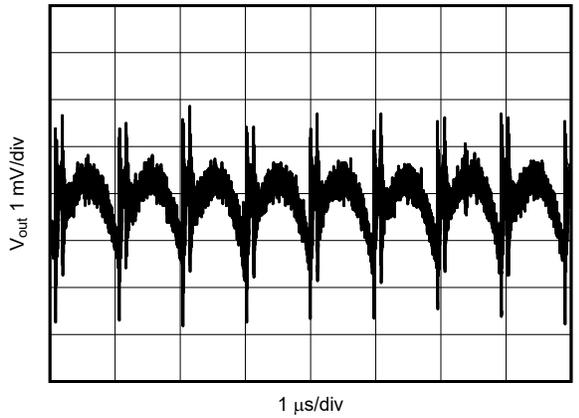
12 V to 1.2 V, 1 A    2.2  $\mu\text{H}$ , 1 MHz    First L-C Only
