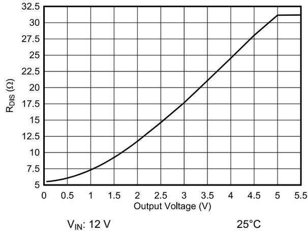
Figure 6-43. Output Discharge Resistance vs Output Voltage
