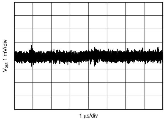
12 V to 1.2 V, 1 A    2.2  $\mu\text{H}$ , 1 MHz    First and second L-C
