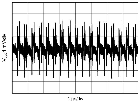
12 V to 3.3 V, 1 A 2.2  $\mu\text{H}$ , 2.2 MHz First L-C Only
