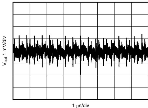
5 V to 1.8 V, 1 A 2.2  $\mu\text{H}$ , 2.2 MHz First L-C Only
