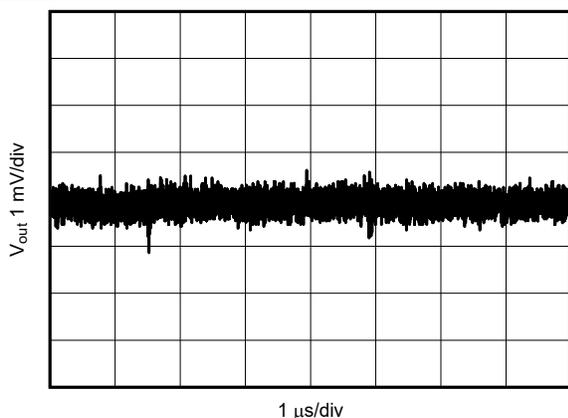
12 V to 3.3 V, 1 A 2.2  $\mu\text{H}$ , 2.2 MHz First and second L-C
