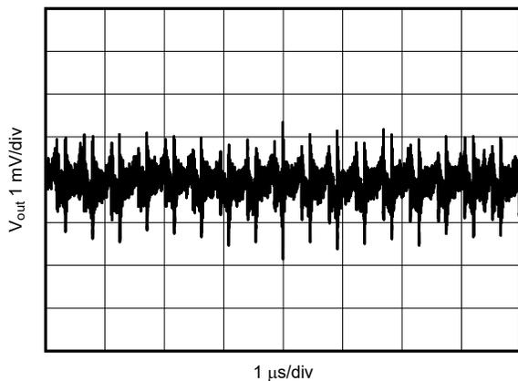
5 V to 3.3 V, 1 A 2.2  $\mu\text{H}$ , 2.2 MHz First L-C Only
