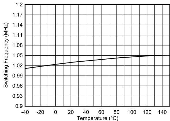
**Figure 6-40. Oscillator Frequency vs Temperature**
