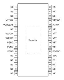
Figure 5-1. DAP Package, 32-Pin HTSSOP (Top View)
