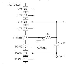
Figure 8-2. RC Filter for VTTSNS
