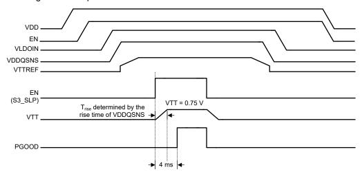
Figure 8-4. Typical Timing Diagram of Tracking Startup and Shutdown
