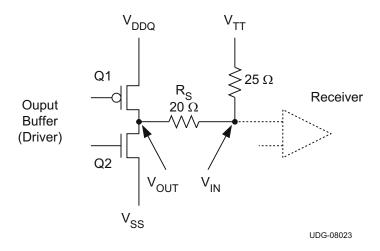
Figure 8-6. DDR Physical Signal System SSTL Signaling
