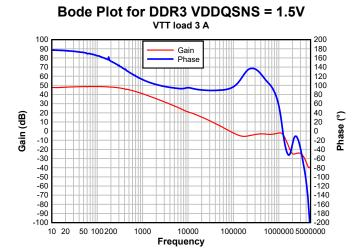
Figure 8-7. Bode Plot for a Typical DDR3 Configuration
