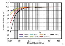
Figure 8-5. Current Efficiency vs I<sub>OUT</sub> and Temperature
