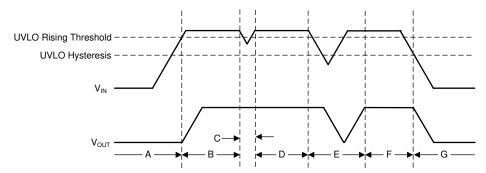
Figure 8-2. Typical UVLO Operation
