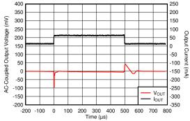
Load Transient Response ( $V_{IN} = V_{OUT} + 1 V$ ,  $C_{OUT} =$ 1  $\mu$ F, I<sub>OUT</sub> = 1 mA to 50 mA in 1  $\mu$ s)
