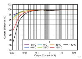
**Ground Current Efficiency vs Output Current**
