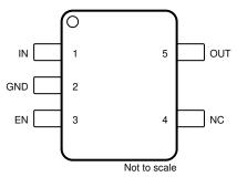
Figure 5-2. DBV Package, 5-Pin SOT-23 (Top View)
