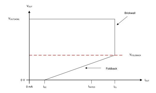
Figure 7-1. Foldback Current Limit
