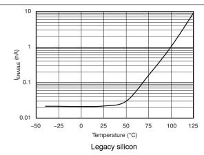
Figure 5-45. I<sub>ENABLE</sub> vs Temperature
