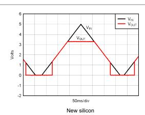
Figure 5-44. TPS73701-Q1, V<sub>OUT</sub> = 3.3V Power-Up and Power-Down
