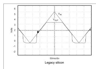
Figure 5-43. TPS73701-Q1, V<sub>OUT</sub> = 3.3V Power-Up And Power-Down
