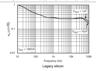
Figure 5-27. Noise Spectral Density
