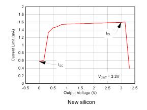
Figure 5-17. Current Limit vs V<sub>OUT</sub> (Foldback)
