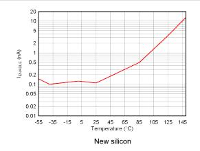
Figure 5-46. I<sub>EN</sub> vs Temperature
