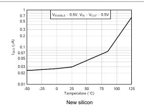
Figure 5-15. Ground Pin Current In Shutdown vs Temperature
