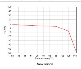
Figure 5-48. TPS73701-Q1  $I_{FB}$  vs Temperature
