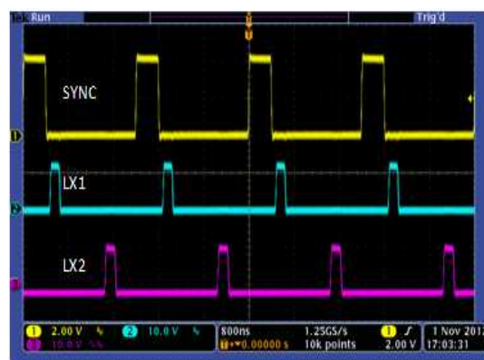
Figure 31. Synchronization at 500 kHz
