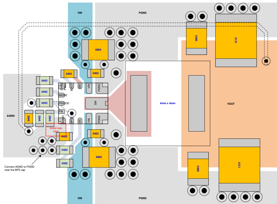
Figure 10-1. Example PCB Layout
