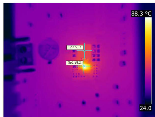
Figure 6-14. Thermal Image at 14-A Output Current
