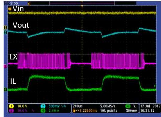
Figure 8. Load Transient
