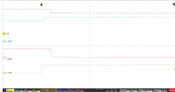
Figure 9-6. State Transition From LPM to Active Mode ( \overline{\text{LPM}} = Low to High, V_{\text{IN}} = 48V, No Load)
