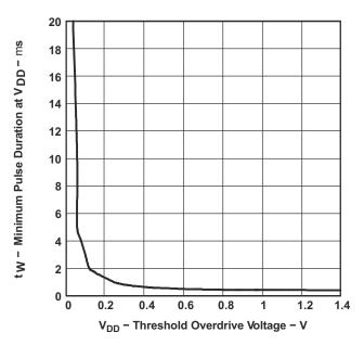
Figure 8-2. Minimum Pulse Duration at V<sub>DD</sub> vs V<sub>DD</sub> Threshold Overdrive Voltage
