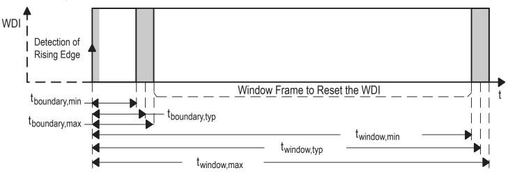
Figure 7-2. Upper and Lower Boundary Visualization
