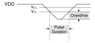
Figure 7-1. Overdrive Versus Pulse Duration
