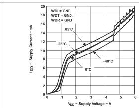
Figure 6-2. Supply Current vs Supply Voltage
