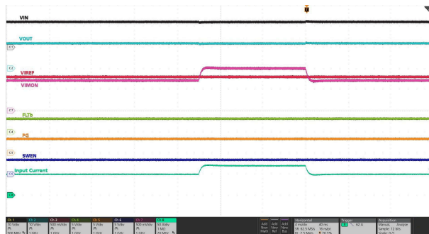
Figure 7-49. Power Good Assertion
