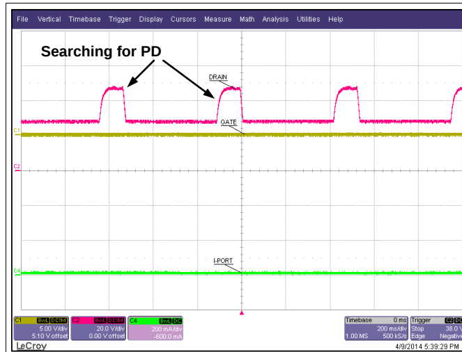
Figure 51. Open Circuit Detection
