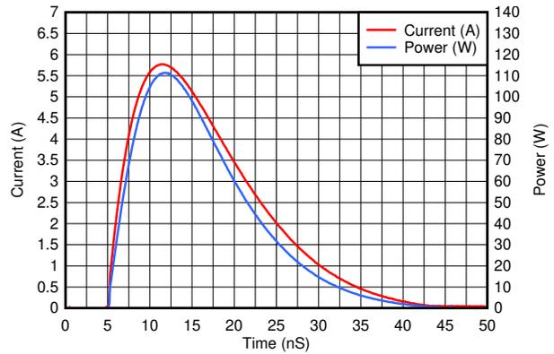
Figure 6-6. Positive Surge Waveform 8/20  $\mu$ s
