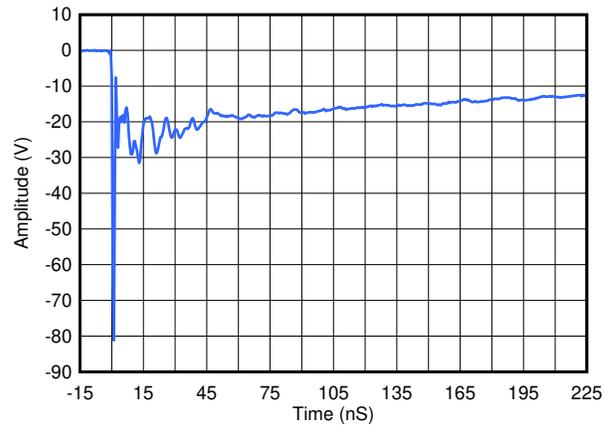
Figure 6-2. ESD Clamp Voltage -8-kV Contact ESD
