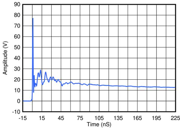
Figure 6-1. ESD Clamp Voltage 8-kV Contact ESD
