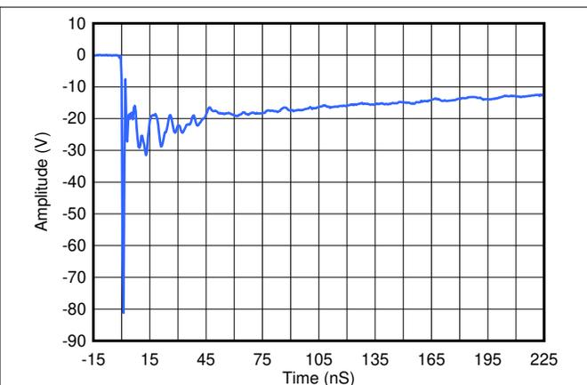
**Figure 8-3. ESD Clamp Voltage –8-kV Contact ESD**
