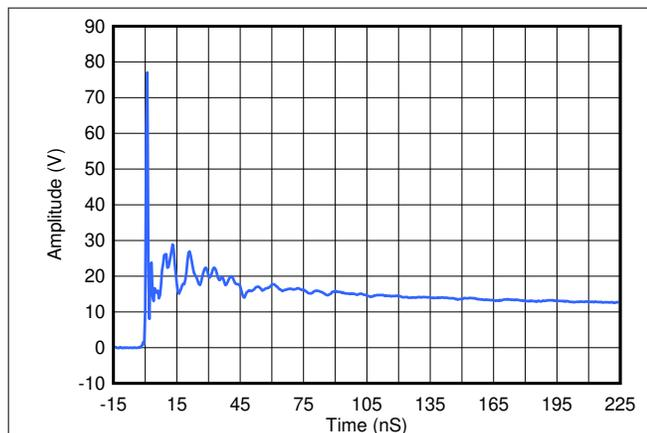
**Figure 8-2. ESD Clamp Voltage 8-kV Contact ESD**
