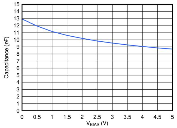
Figure 6-8. Pin Capacitance Across V<sub>BIAS</sub>
