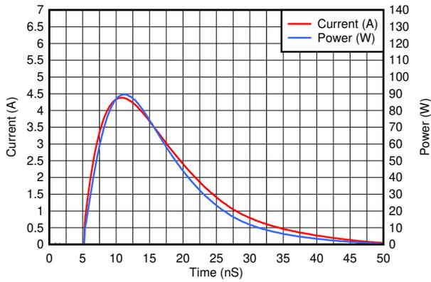
Figure 6-7. Negative Surge Waveform 8/20  $\mu$ s
