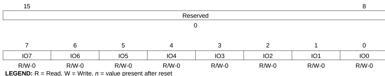
Figure 3-21. General-Purpose I/O Status Register (GPIOSR) [MMR Address 003Dh]
