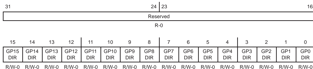
Figure 19. GPIO Direction Register (GPDIR) [Hex Address: 01B0 0004]
