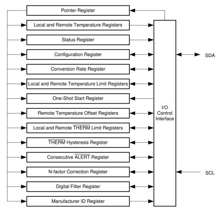
Figure 7-6. Internal Register Structure
