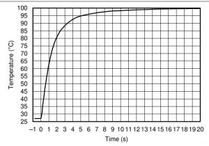
Figure 8-4. Temperature Step Response
