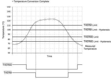
Figure 7-3. THERM and THERM2 Interrupt Operation
