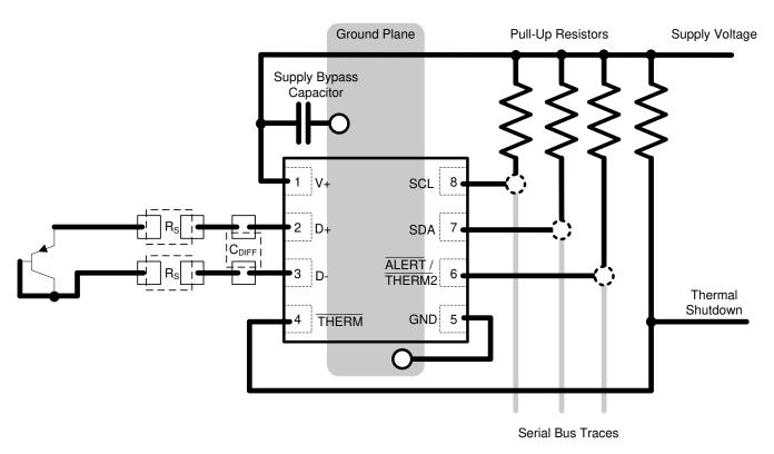
Figure 10-2. TMP451-Q1 Layout Example
