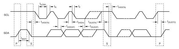
Figure 6-1. Two-Wire Timing Diagram
