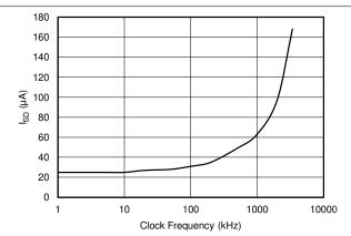
Figure 6-9. Shutdown Quiescent Current vs. SCL Clock Frequency
