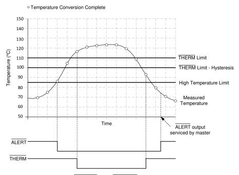
Figure 7-2. ALERT and THERM Interrupt Operation
