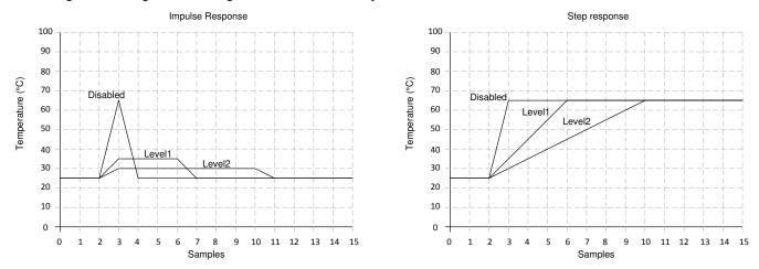
Figure 7-1. Filter Response to Impulse and Step Inputs
