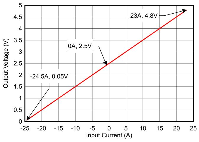
Figure 9-4. Application Example Design Transfer Curve
