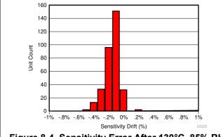
Figure 8-4. Sensitivity Error After 130°C, 85% RH HAST
