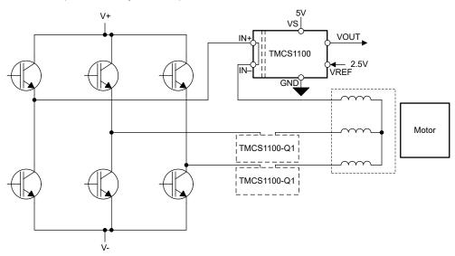
Figure 9-2. Inline Motor Phase Current Sensing
