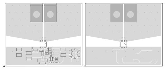
Figure 9-7. Recommended Board Top (Left) and Bottom (Right) Plane Layout
