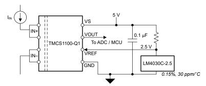
Figure 9-3. TMCS1100 Example Current-Sense System Design
