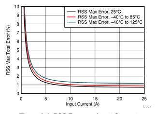
Figure 9-1. RSS Error vs. Input Current
