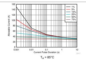
Figure 7-7. Maximum Repetitive Pulsed Current vs. **Pulse Duration**
