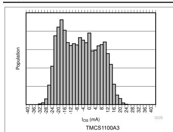
Figure 6-7. Input Offset Current Production Distribution
