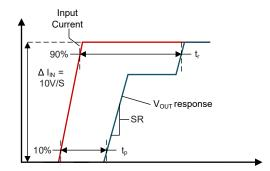
Figure 7-4. Current Overload Transient Response
