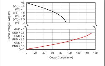
Figure 6-12. Output Swing vs Output Current
