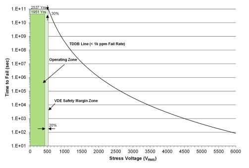
Figure 8-1. Insulation Lifetime
