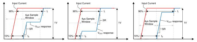
Figure 7-3. Small Current Input Step Transient Response
