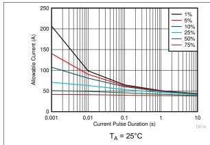
Figure 7-6. Maximum Repetitive Pulsed Current vs. **Pulse Duration**
