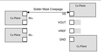
Figure 9-6. Layout for System Creepage Requirements
