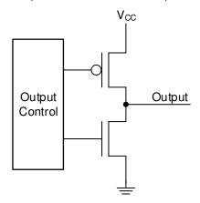
Figure 8-4. Push-Pull Output (Simplified)
