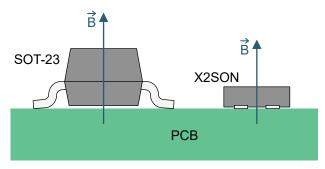
Figure 8-1. Direction of Sensitivity
