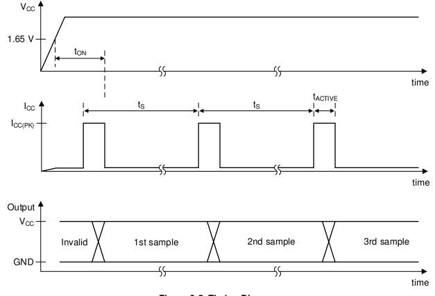
Figure 8-5. Timing Diagram
