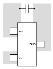
Figure 9-14. SOT-23 Layout Example
