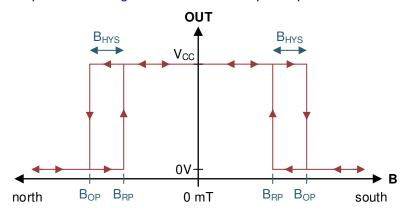
Figure 8-3. Omnipolar Functionality
