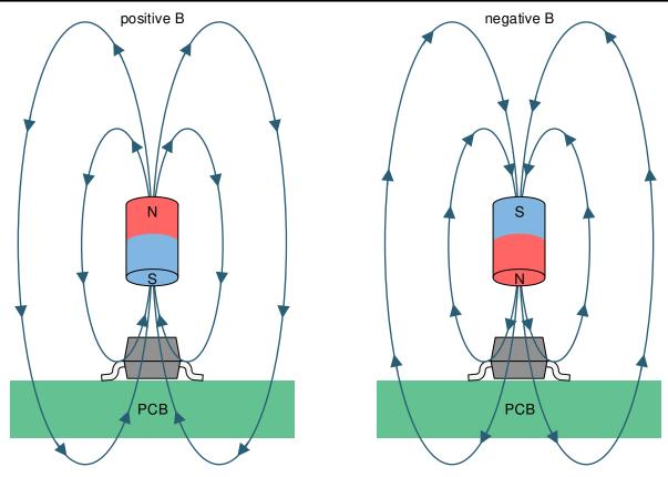
Figure 8-2. Flux Direction Polarity
