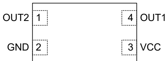
Figure 5-1. ZFC Package 4-Pin X1LGA Top View
