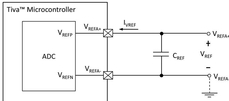
Figure 22-19. ADC Input Equivalency Diagram
