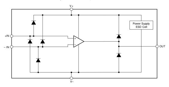
Figure 8-5. Equivalent Internal ESD Circuitry
