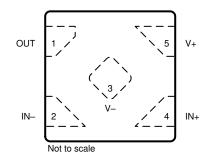
Figure 6-4. TLV9041 DPW Package 5-Pin X2SON Top View
