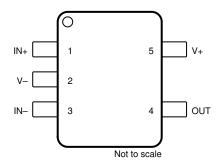
Figure 6-2. TLV9041U DBV Package 5-Pin SOT-23 Top View
