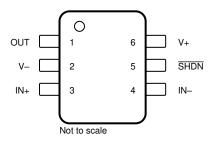
Figure 6-5. TLV9041S DBV Package 6-Pin SOT-23 Top View
