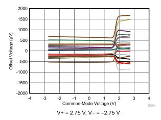
Figure 8-1. TLV904x Offset Voltage vs Common-Mode
