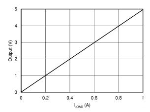
Figure 9-2. Low-Side, Current-Sense Transfer Function
