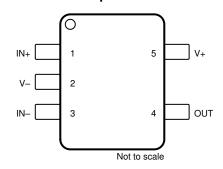
Figure 6-3. TLV9041 DCK Package 5-Pin SC70 Top View
