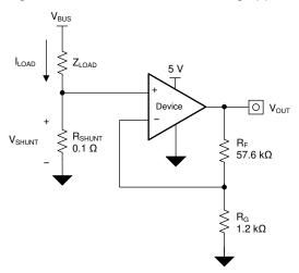
Figure 9-1. TLV904x in a Low-Side, Current-Sensing Application
