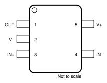
Figure 6-1. TLV9041 DBV Package 5-Pin SOT-23 Top View
