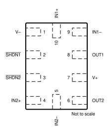
Figure 6-8. TLV9042S RUG Package 10-Pin X2QFN Top View
