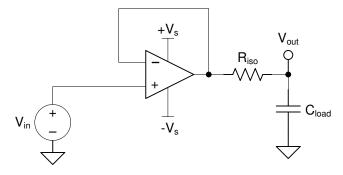
Figure 8-3. Improving Capacitive Load Drive
