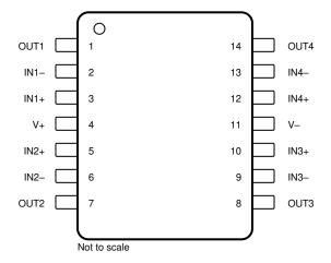
Figure 6-9. TLV9044 D, PW and DYY Packages 14-Pin SOIC, TSSOP and SOT-23 Top View
