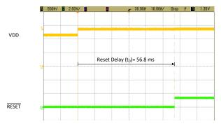
Figure 9-5. TLV840EVM RESET Time Delay (t<sub>D</sub>) with 0.1-µF Capacitor
