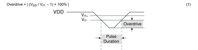
Figure 8-2. Overdrive vs Pulse Duration
