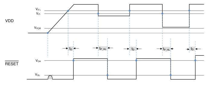
(3)  $\overline{RESET}$  output is undefined when  $V_{DD}$  is <  $V_{POR}$  and limited to  $V_{OL}$  for  $V_{DD}$  slew rate = 100mV /  $\mu S$
