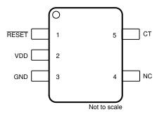
Figure 6-1. Pin Configuration TLV840C, DBV Package, 5-Pin SOT-23, TLV840C Top View
