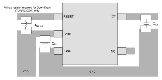
Figure 11-1. TLV840C Recommended Layout
