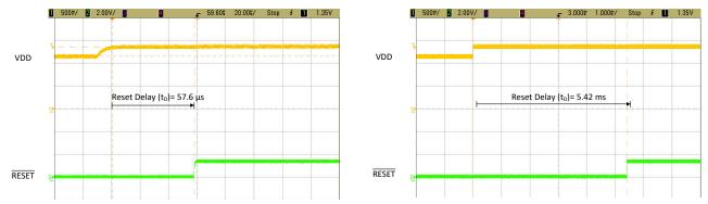
Figure 9-3. TLV840EVM RESETTime Delay (t<sub>D</sub>) with Figure 9-4. TLV840EVM RESETTime Delay (t<sub>D</sub>) with No Capacitor 0.01-µF Capacitor
