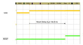
Figure 9-5. TLV840EVM RESET Time Delay (t<sub>D</sub>) with 0.1-μF Capacitor
