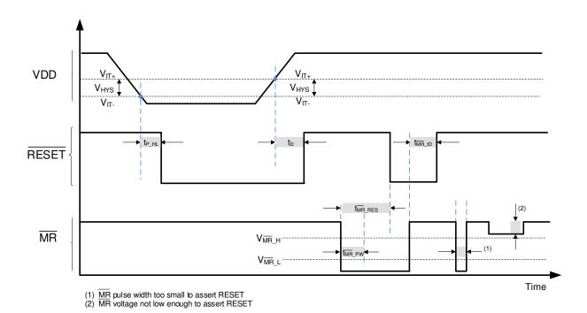
Figure 8-4. Timing Diagram MR and RESET (TLV840M)
