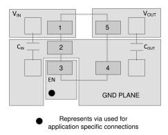
Figure 9-2. SOT-23 Layout Example
