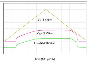
$R_L = 6.2 \Omega$ ,  $V_{EN} = V_{IN}$ , 1- $\mu$ F output capacitor
