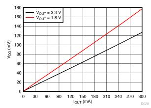
**Dropout Voltage vs Output Current**
