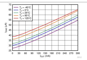
Figure 6-2. Ground Pin Current vs I<sub>OUT</sub> and Temperature
