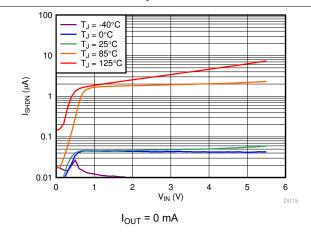
Figure 6-4. Shutdown Current vs V<sub>IN</sub> and Temperature
