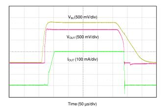
Figure 8-3. 1.8-V to 1.5-V Regulation at 300 mA
