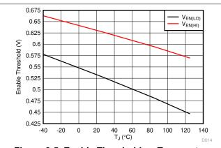
Figure 6-5. Enable Threshold vs Temperature
