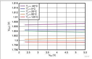
Figure 6-1. 1.8-V Regulation vs V<sub>IN</sub> (Line Regulation) and Temperature
