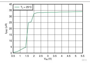
Figure 6-3. Ground Pin Current vs VIN
