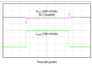
$V_{IN}$  = 2.0 V, 1- $\mu$ F output capacitor, output current slew rate = 0.25 A/µs
