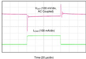
$V_{IN}$  = 3.8 V,1- $\mu$ F output capacitor, output current slew rate = 0.25 A/µs
