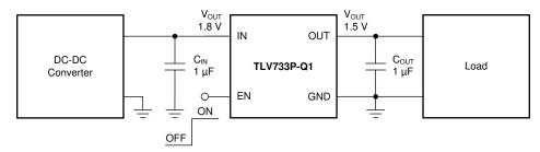
Figure 8-2. DC-DC Converter Post Regulation
