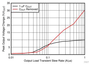
Output current stepped from 50 mA to 300 mA, output voltage change measured at positive dl/dt
