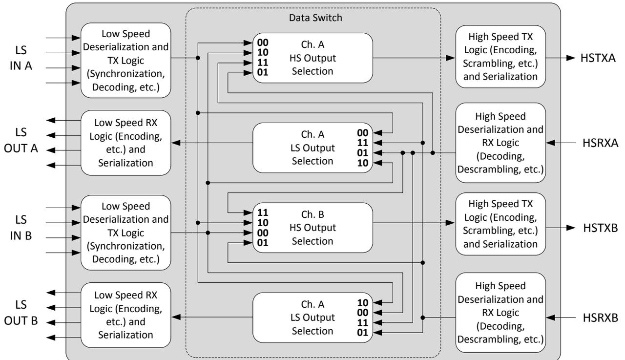
Figure 7-1. Signal Routings for Integrated Smart Switch
