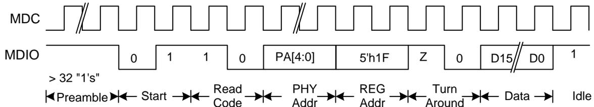
Figure 7-14. CL22 - Indirect Address Method – Data Read
