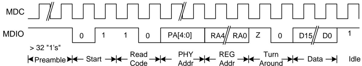
Figure 7-9. CL22 - Management Interface Read Timing
