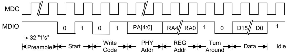
Figure 7-10. CL22 - Management Interface Write Timing
