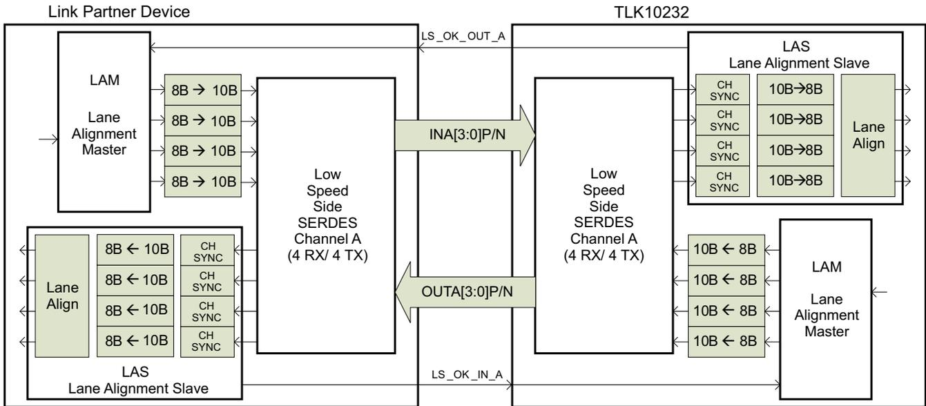
Figure 5-2. Block Diagram of the Lane Alignment Scheme
