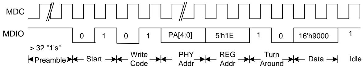
Figure 7-13. CL22 - Indirect Address Method – Address Write
