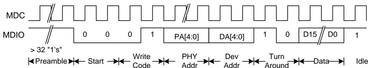
Figure 7-6. CL45 - Management Interface Extended Space Write Timing
