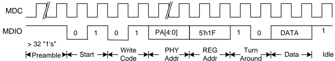
Figure 7-12. CL22 - Indirect Address Method – Data Write
