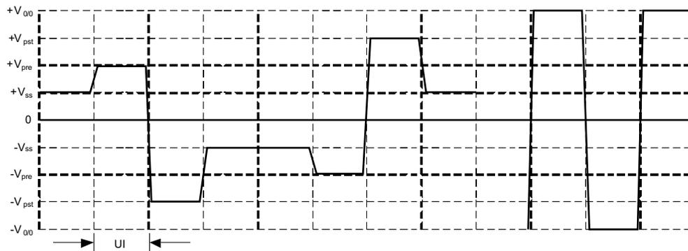
$h_{-1}$  = TWPRE (0%  $\geq$  -17.5% for typical application) setting
