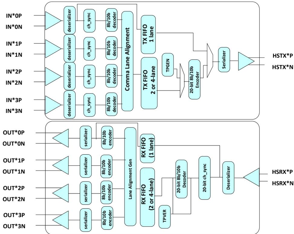
Figure 5-1. Block Diagram Showing General Purpose SerDes Mode
