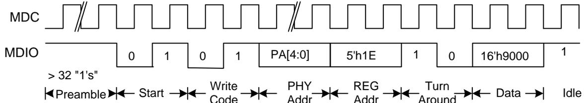
Figure 7-11. CL22 – Indirect Address Method – Address Write
