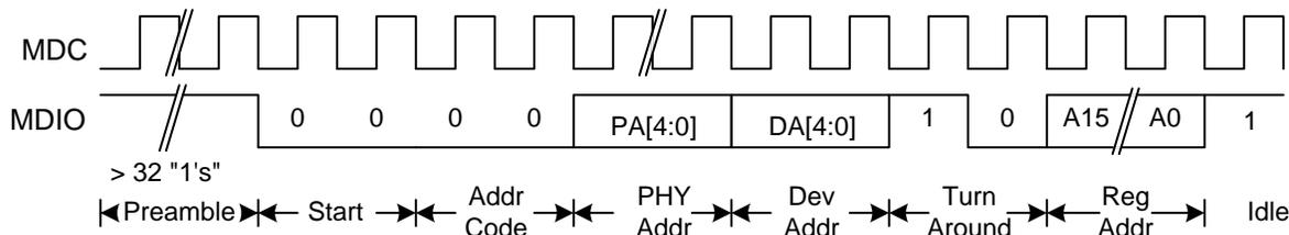
Figure 7-5. CL45 - Management Interface Extended Space Address Timing
