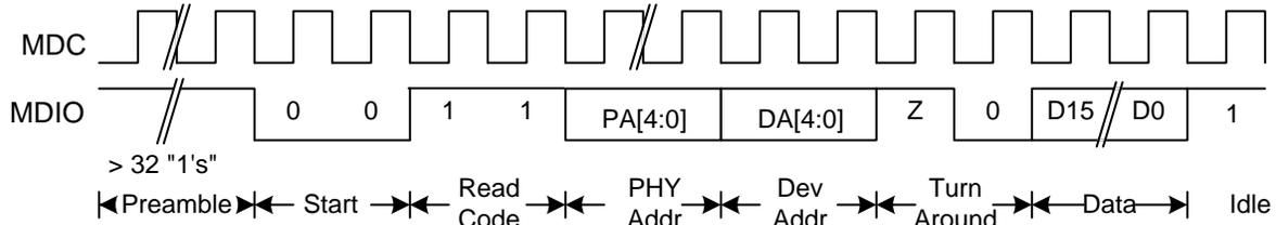
Figure 7-7. CL45 - Management Interface Extended Space Read Timing
