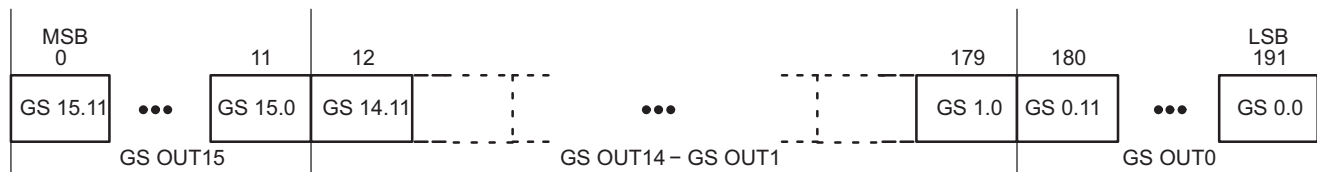
Figure 17. Grayscale Data Packet Format
