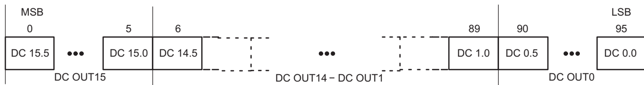
Figure 15. Dot Correction Data Packet Format
